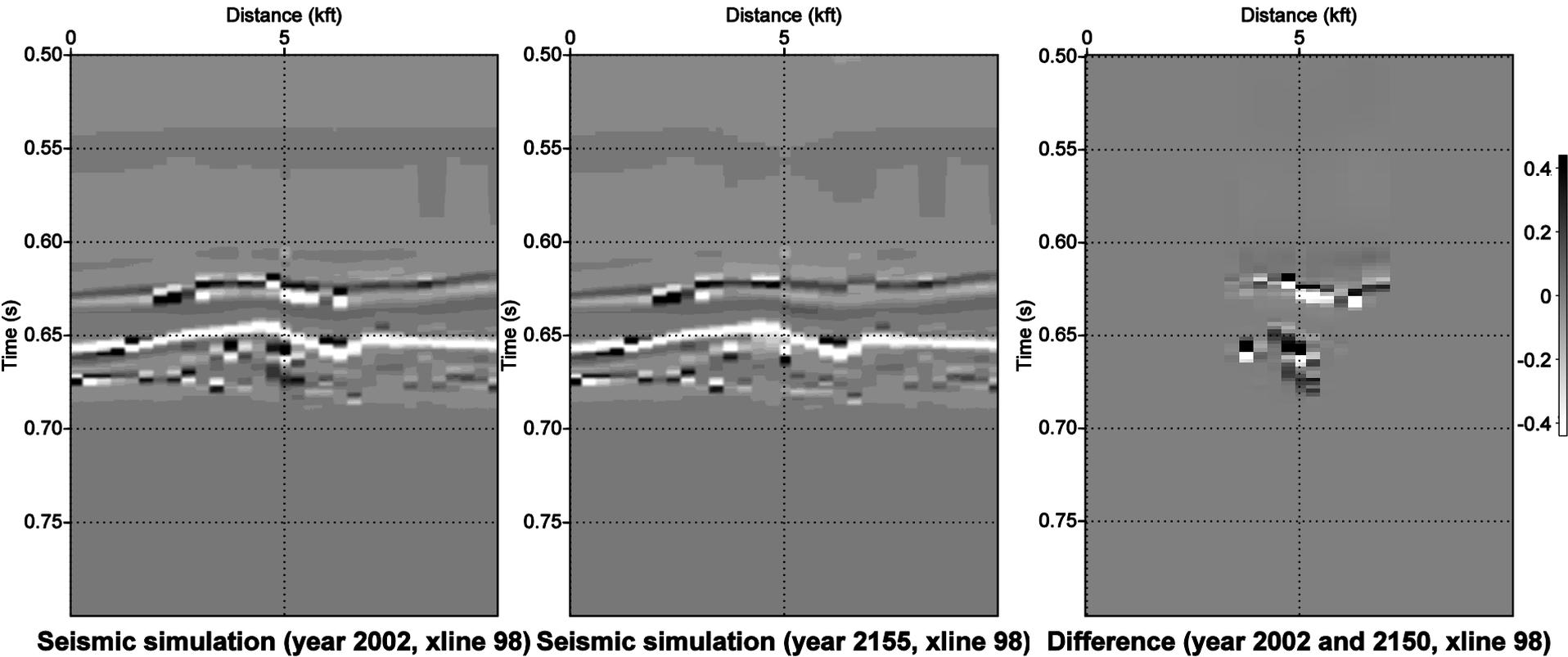
Figure 3b. Seismic data (crossline 98) at the different simulation time (2002' and 2155') and the difference. Displayed from 500ms to 800ms.
