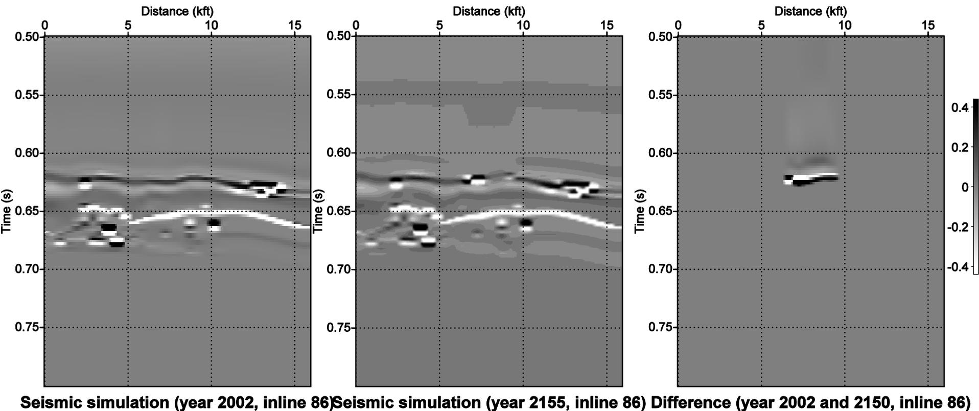
Figure 3a. Seismic data (inline86) at the different simulation time (2002' and 2150') and the difference. Displayed from 500ms to 800ms. It caused 4% impedance change.
