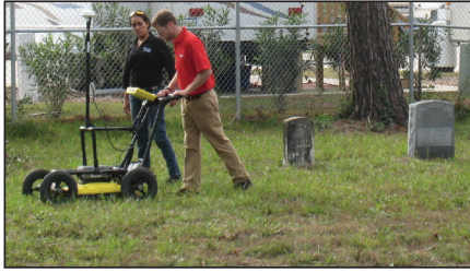
Figure 1: A University of Houston team member (Marcus Zinecker, with Lone Star's Janet Flores) is pushing the Noggin 250 MHz GPR SmartCart over one of the survey grids.
