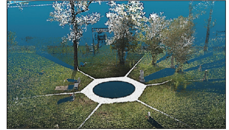
Figure 3: Colorized pointcloud collected with a ground-based LiDAR scanner (located in the center) shows the headstones at the Cemetery.
