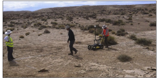
Figure 2: Photo of acquiring GPR data using the 250 MHz Noggin SmartCart System at the Utah survey location.
