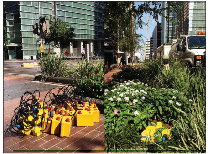
Figure 2: Autonomous seismic nodes (Geospace GSRs) awaiting deployment (left) along Main St. in downtown Houston and then planted (right) for the implosion.
