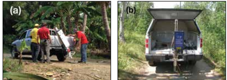
Figure 2: Seismic sources in Haiti: a) Vertical accelerated weight drop source (PEG), b) Slanted accelerated weight drop (GISCO) on the line.
