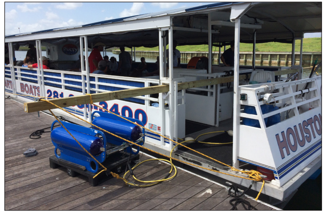
Figure 6: The boomer seismic source rigged from the side of a “Party Boat” out of South Shore Harbor near Kemah. Streamers (hydrophone cables) were attached on arms from the vessel’s stern.
