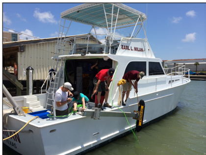
Figure 1: Bathymetric and side-scanning sonar rigged from the side of the research vessel Milan in Galveston Harbor during the 2014 Geophysics Field Camp.
