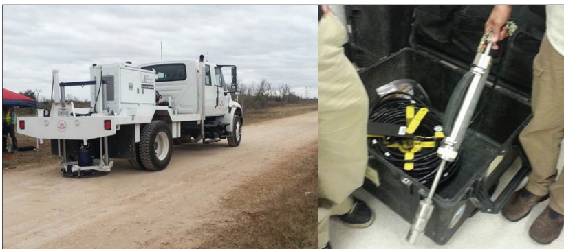
Figure 2: The UH Vibroseis truck and downhole source used for VSP acquisition.
