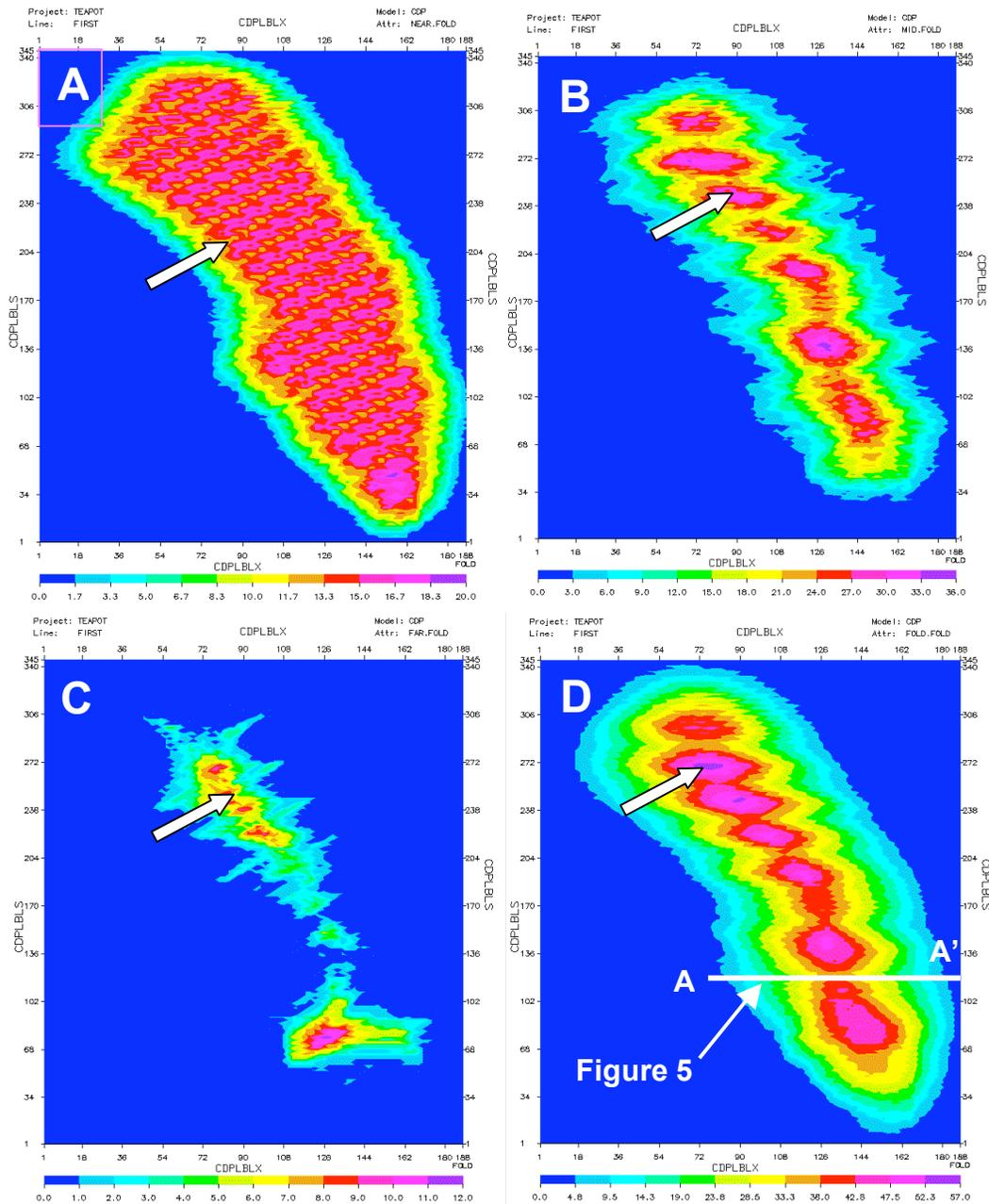
**Figure 3.** Fold analysis of Teapot Dome seismic data. **A.** Near-offset (0-5000 ft.) fold, **B.** Mid-offset (5000-10000 ft.) fold, **C.** Far-offset (10000-18000 ft.) fold, and **D.** Total fold. Maximum fold is 57. Blue color in background is area of zero fold (no data). White arrows point to acquisition footprints that trend EW and N59E and that relate to source and receiver alignments. See Figure 5 for seismic section A-A'.
