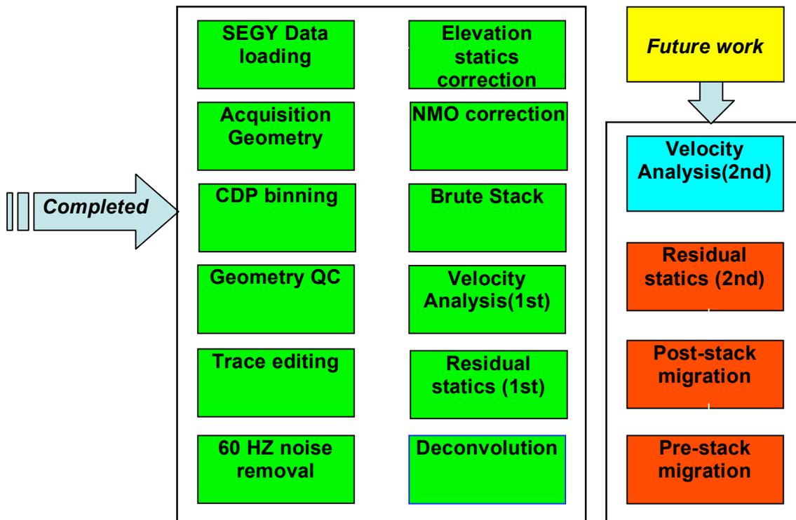
**Figure 6.** Processing workflow for prestack migration of Patoka 3-D seismic survey. Work has been completed through the deconvolution step (green boxes). Velocity analysis is in progress (blue box). Application of residual static corrections and the migration of the data are the final steps to be done (red boxes).
