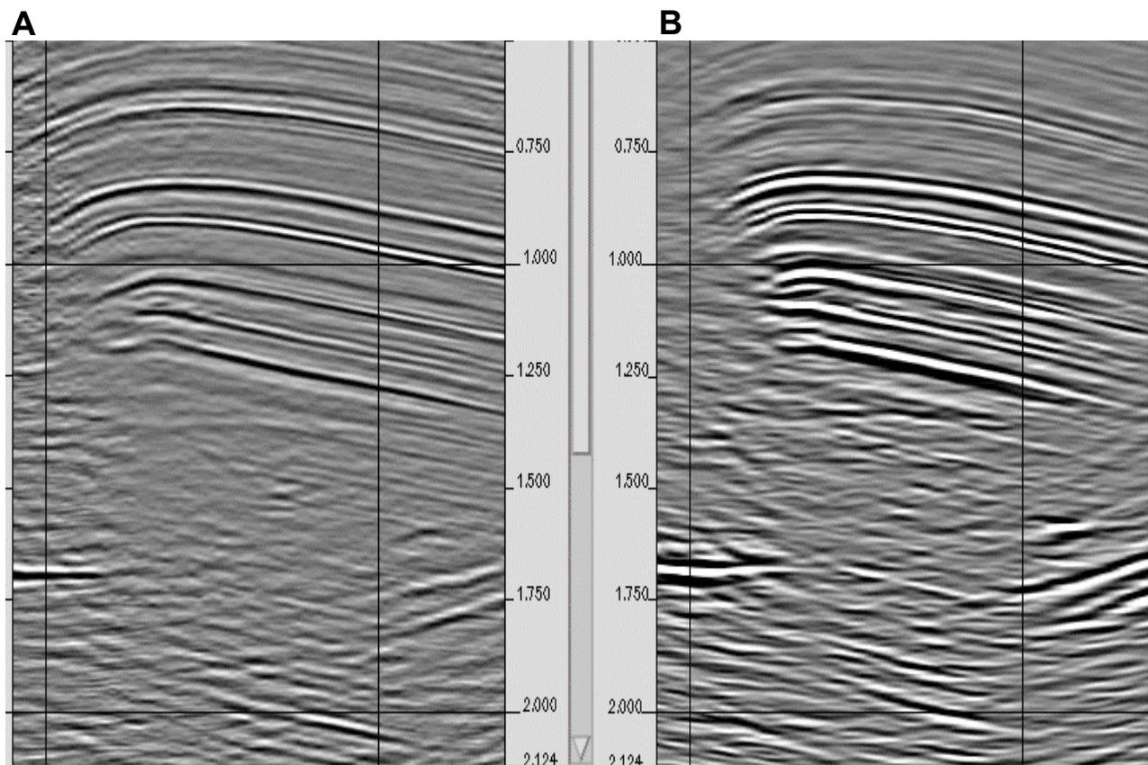
**Figure 5.** Comparison of pre-stack time migrated subline 120 at Teapot Dome (Section A-A' on Figure 3). **A.** Profile from RMOTC processed pre-stack time migrated seismic data volume. **B.** Profile from UH processed pre-stack time migrated seismic data volume.
