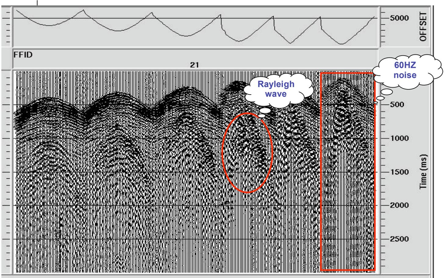
**Figure 7.** Six shot gathers from the Patoka seismic survey (TWT vs offset distance). Rayleigh waves or ground roll and 60HZ noise are evident throughout the survey.
