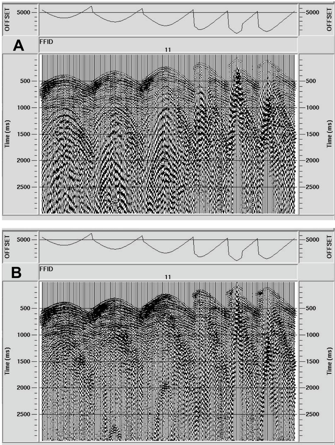
**Figure 9.** 228-channel shot gather from the Patoka survey showing results of filtering to remove ground roll. **A.** Original data with ground roll (compare with Figure 7). **B.** Figure 4A after removal of ground roll with an Ormsby low-cut filter (8-10-200-240)
