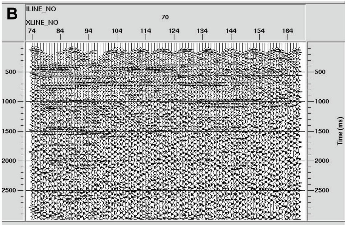
**Figure 10.** Comparison of inline 70 before and after deconvolution. **A.** Stack after residual statics correction. **B.** Stack after residual statics and predictive deconvolution. A possible basement structure is evident between lines 104-164 at the TWT interval of 2.0-2.5 sec.
