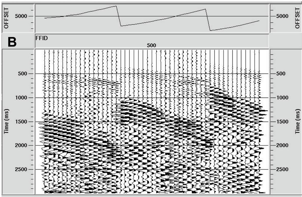
**Figure 8.** Three shot gathers from the Patoka survey (TWT vs offset distance) showing results of filtering to remove 60HZ noise. Each gather contains all of the traces from a single shot. **A.** Original data with 60HZ noise (compare with Figure 7). **B.** Data after removal of 60HZ noise with a 60HZ notch filter showing improved reflector continuity.
