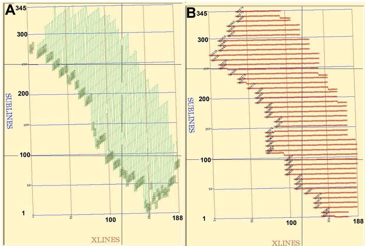
**Figure 2.** Seismic coverage of Teapot Dome field. **A.** Shot locations (green dots). **B.** Receiver locations (red dots). The line spacing is 110 feet by 110 feet.
