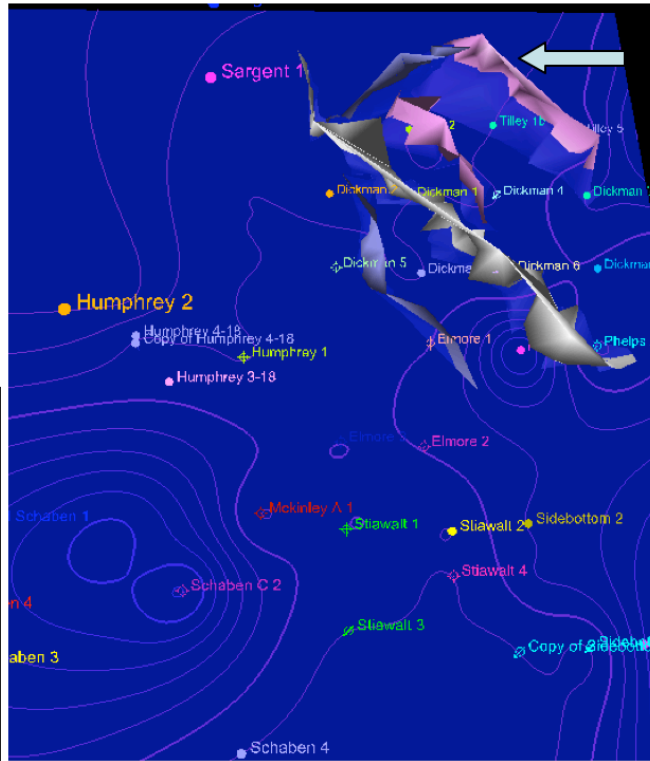
Figure 1-7b. Extracted ANT planes with dip > 45°. One 4000 ft long NE plane (arrow) was extracted from both passive and aggressive ANT volumes.
