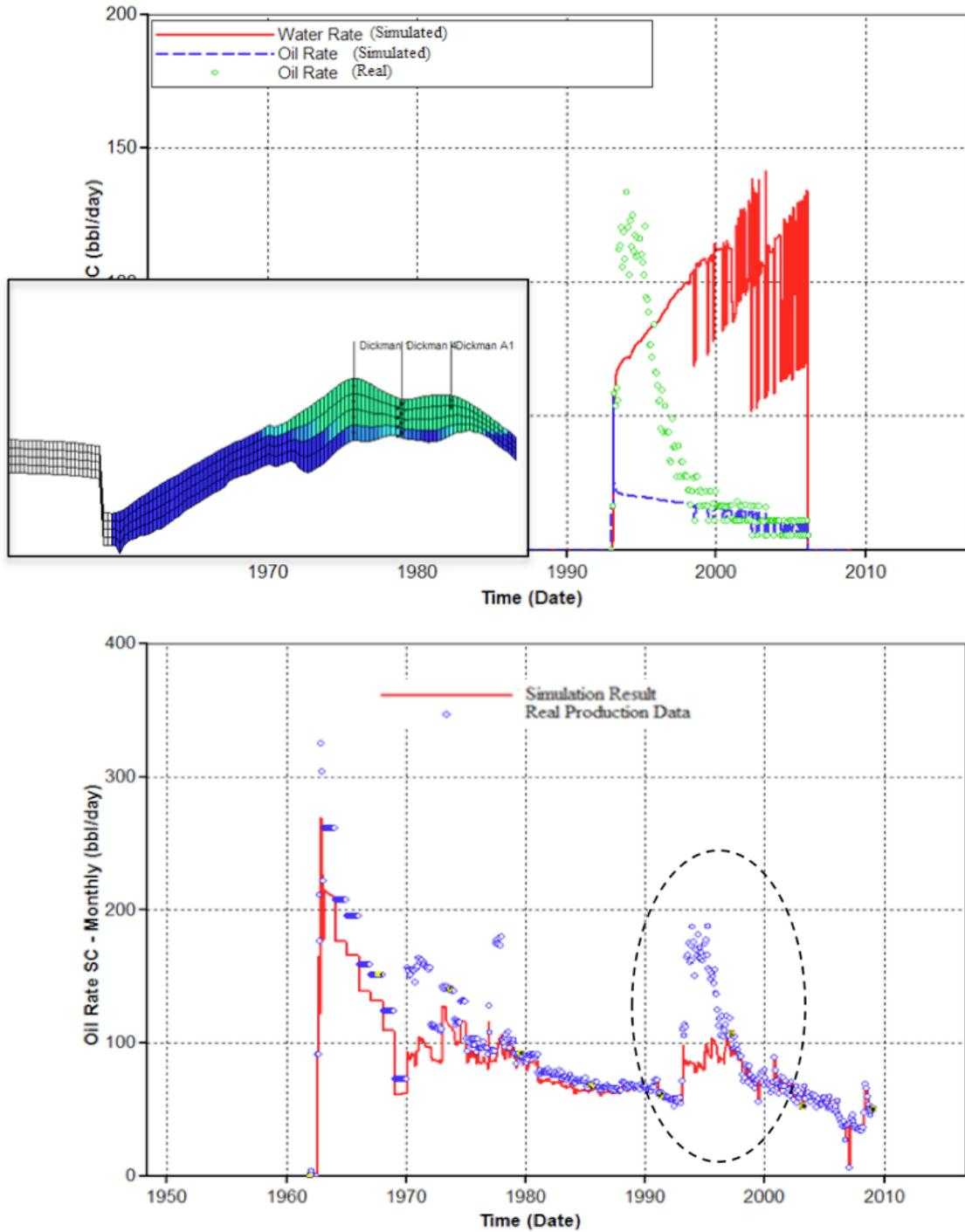
Figure 8: Upper: Simulation result for Dickman A1 for all production years (1993-1998) using perforations in only the two top simulation layers. The simulated oil production rate (dash blue line) is much lower than the real rate (green dots). Lower: Dickman field total oil production rate shows significant mismatch in the 1993-1998 time period resulting from errors with the Dickman A1 well.
