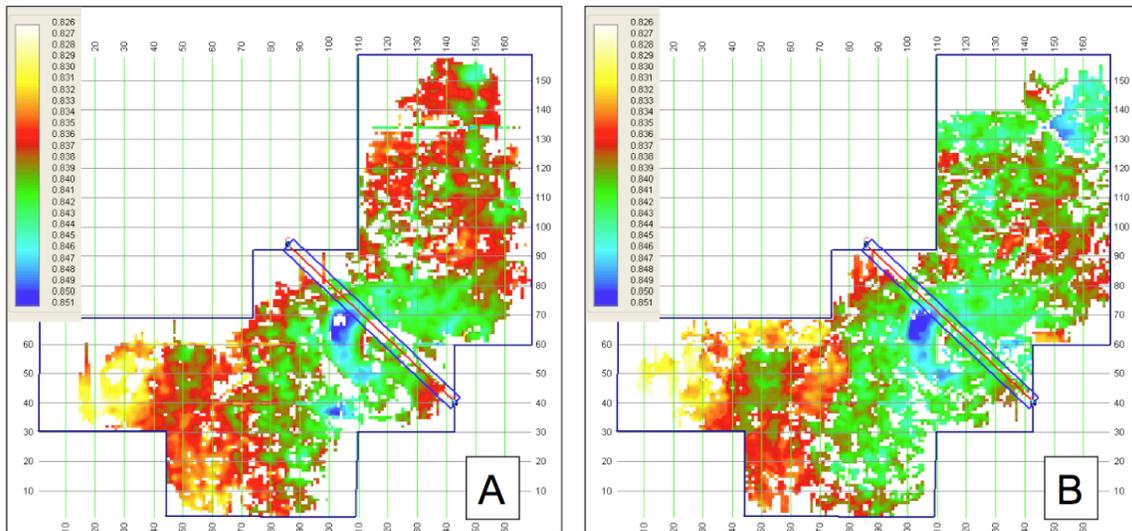
Figure 2. Top Mississippian time structure maps. (A) Tracking result using zero crossing in the amplitude volume. (B) Tracking result using peak in spice volume. Note improved continuity on this irregular, karst surface in the spice-generated map.
