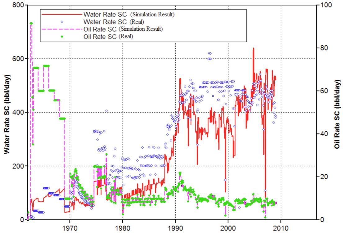
Figure 7: History matching results for Dickman 1 production well (1962- 2009). A good match on oil and water production rate was obtained here.
