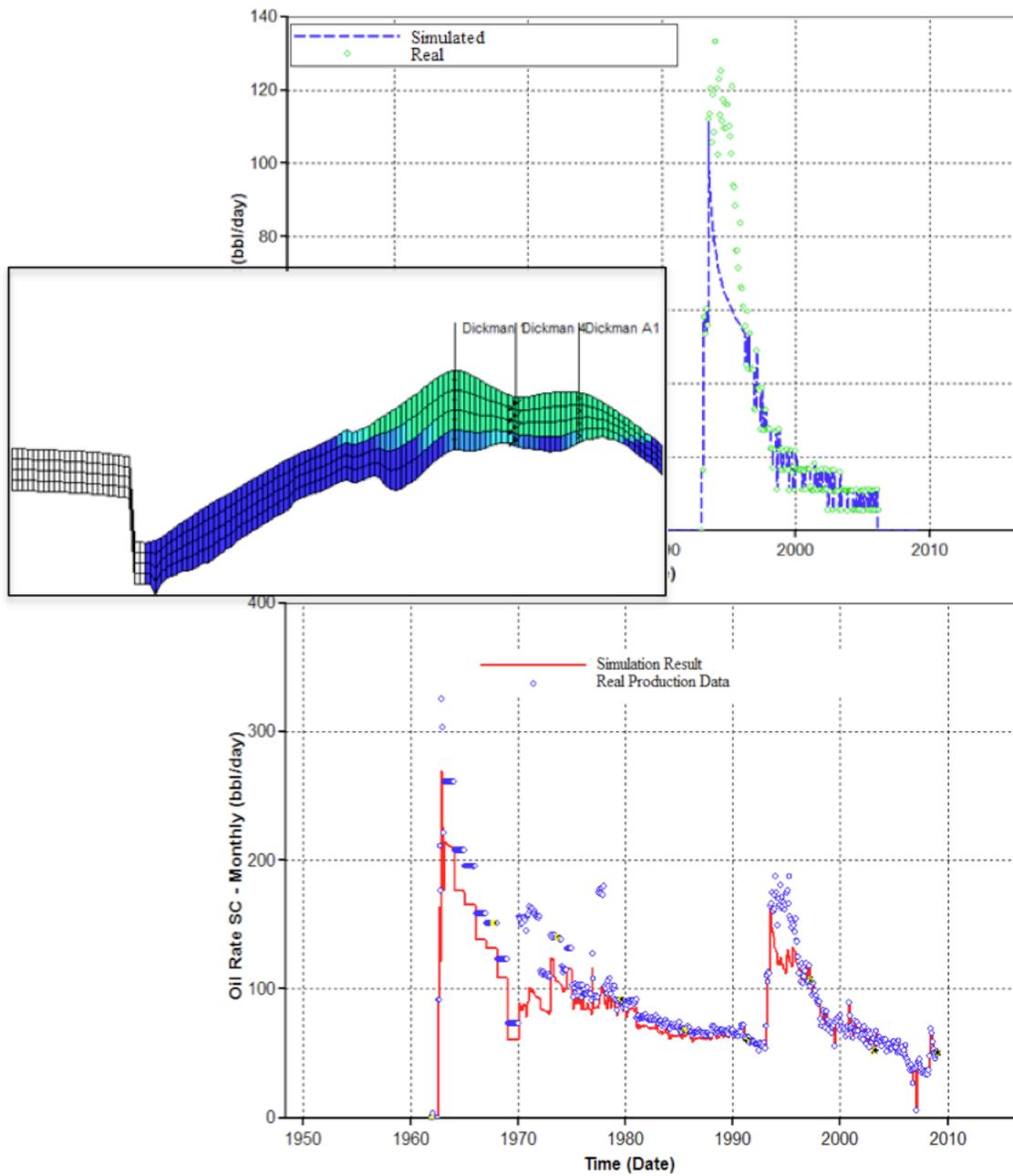
Figure 9. Upper: Improved match for oil production rate at Dickman A1 well after all four simulation layers are assumed to be perforated. Lower: Dickman field total daily oil production rate shows an improved match after all four simulation layers are perforated at the Dickman A1 well. To achieve this match, it was necessary to assume the Dickman A1 well had total depth six feet deeper than the reported value, or there was communication between the simulation layers.
