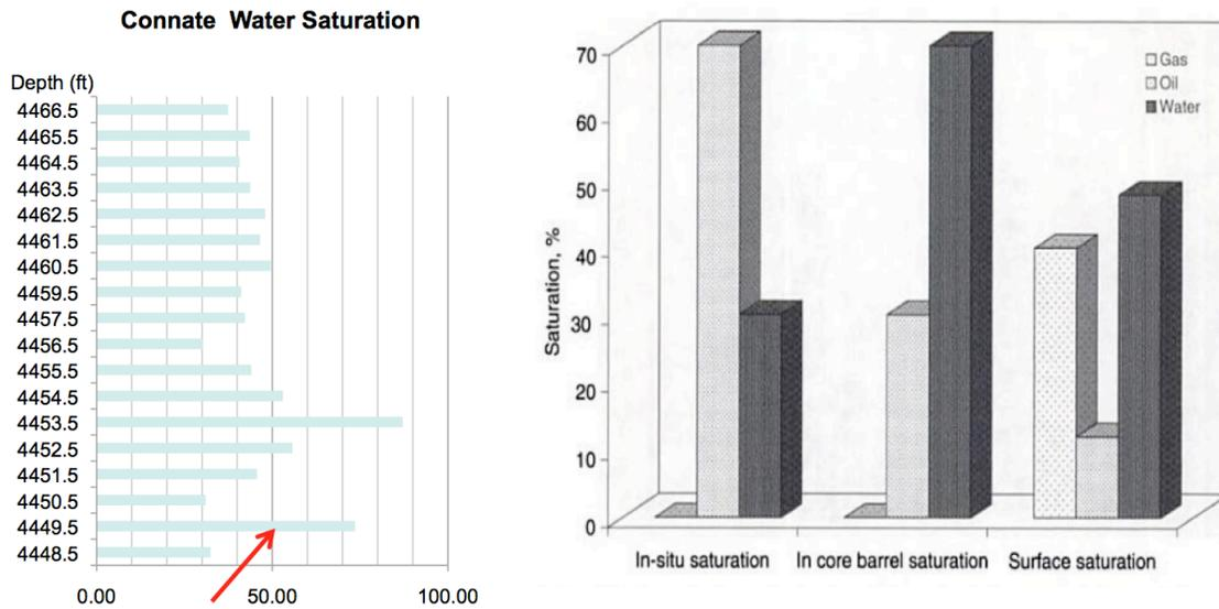
Figure 4. Left: Water saturation from Dickman 2 well core measurement (other wells show similar range of water saturation). Right: Typical alterations in the fluid saturations of a core sample from virgin productive formation that was badly flushed with water-based drilling mud (from Dandekar, 2006). A 70% water saturation measured from flushed cores corresponds to 30% in-situ water saturation.
