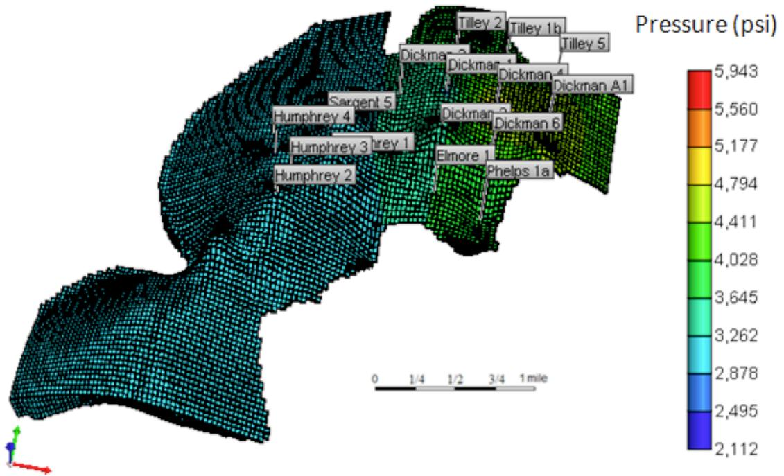
Figure 10. Final reservoir pressure at the end of the history match simulation run.
