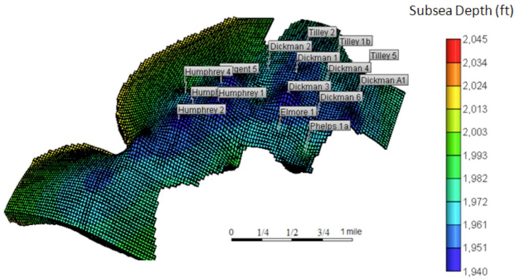
Figure 6: History matching flow simulation grid showing all 15 production wells and the Dickman 4 injection well.
