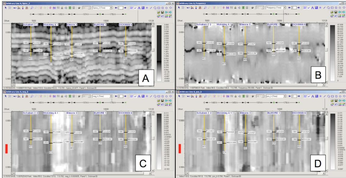
Figure 3. Relationship of spice to other attributes in vertical view along line in Fig 2. (A) Spice; (B) Instantaneous frequency; (C) Negative curvature; (D) Positive curvature.
