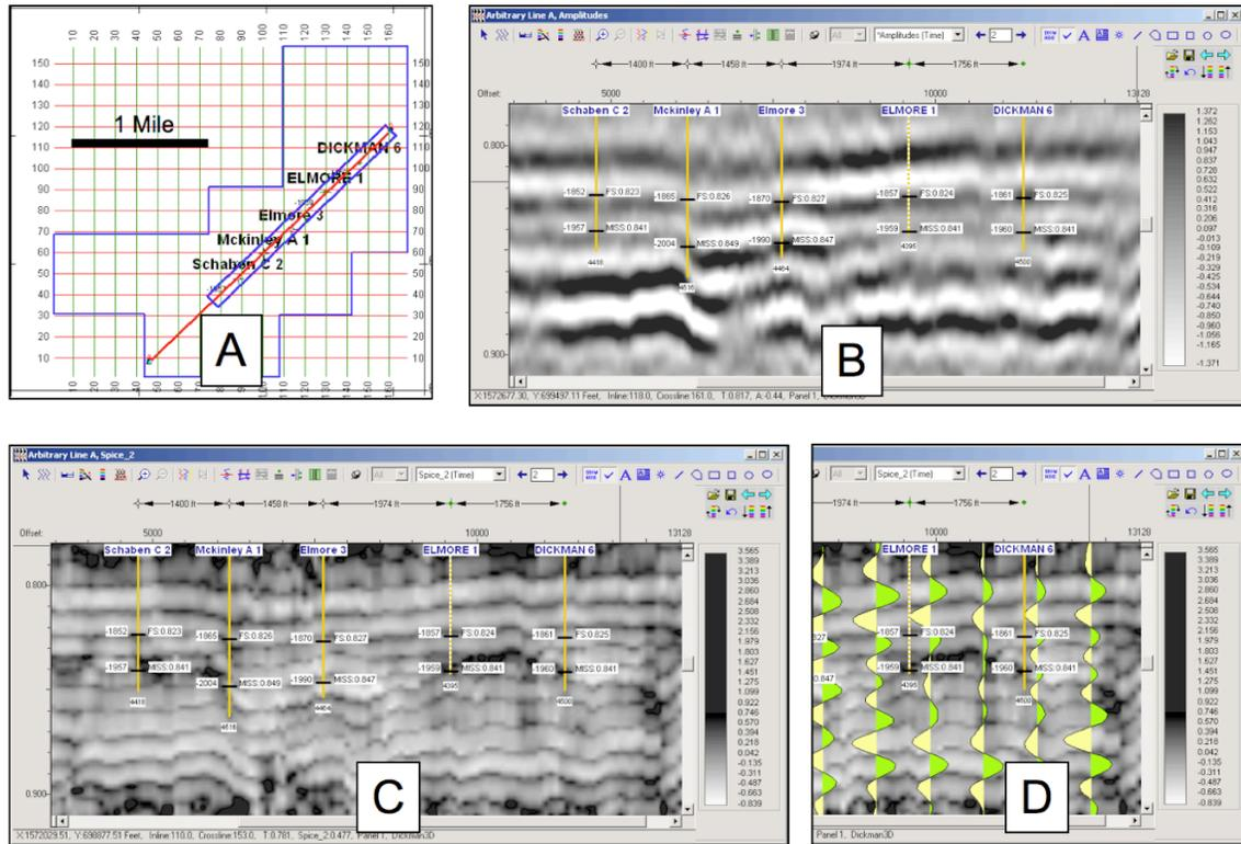
Figure 1. Relationship between seismic amplitude and spice data. A) Base map showing vertical seismic line through selected wells. B) Amplitude section and formation tops. C) Spice data with tops. D) Spice data with amplitude wiggle trace overlay.
