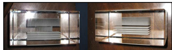
Figure 2. Two further glass models with laser-etched interior fracture zones simulating VTI and HTI regions.
