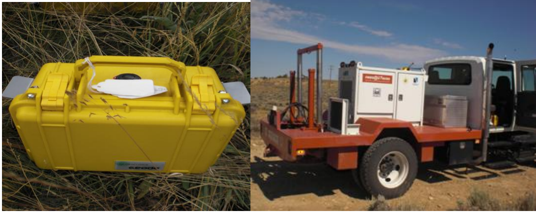
Figure 2-6: Left: Geode (24-channel seismic recording instrument); Right: Vibroseis truck from the NEES, facility in Austin, Tx.
