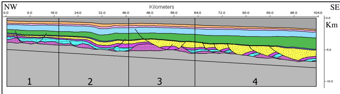
**Figure 24:** In order to restore the whole line, it was necessary to divide the line into four regions and restore each region separately, and then, put the regions together and confirm they could be reconstructed as a whole. Vertical exaggeration is 2:1. All units are in kilometers. Refer to Figure 23 for stratigraphic column.
