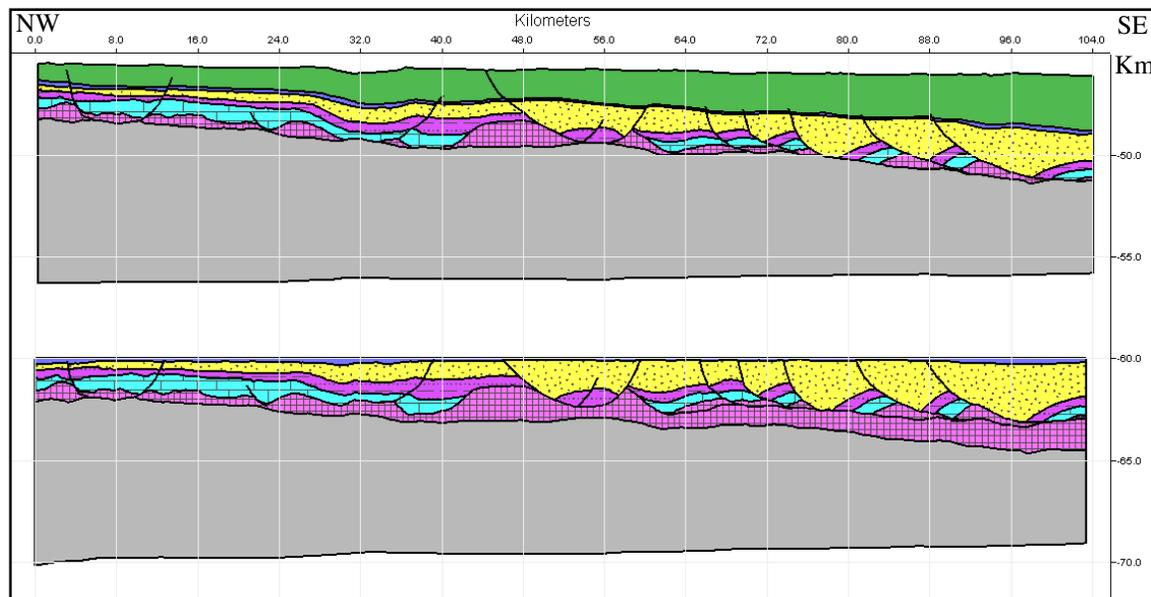
**Figure 28:** After reconstructing the Upper Jurassic, it appears that there was about a 0.4 kilometers of extension between the Upper Jurassic and Pettet. This could be due to salt withdrawal and reactivation along the listric faults to the southeast. Vertical exaggeration is 2:1. Refer to Figure 23 for stratigraphic column. All units are in kilometers.
