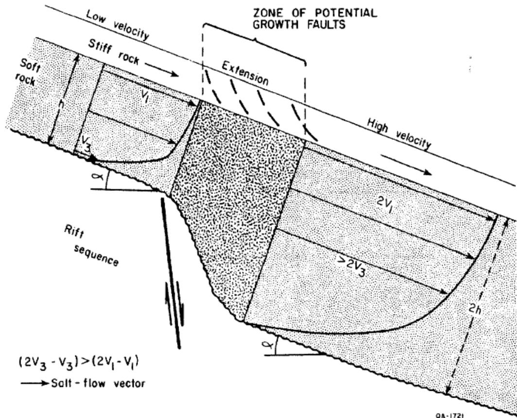
**Figure 14:** Illustration showing the development of a zone of extension due to a stiff glide sheet over an uneven thickness of a soft glide zone such as salt. As the soft glide zone flows faster the stiff overburden is strained and pulled apart resulting in normal faulting. This model could easily represent a salt body overlain by a carbonate system (Jackson and Galloway, 1984).
