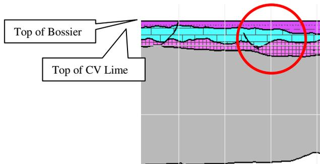
After reconstruction, it appears that dip in reflectors was due to beds forming a syncline in response to salt withdrawal in the area and does not represent the shelf edge.
