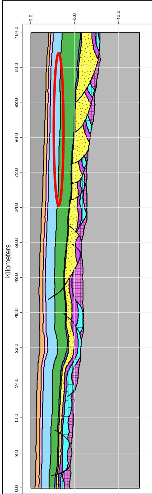
**Figure 44:** Small synform suggesting that salt withdrawal had taken place, but there is recovery and it almost reaches the regional elevation to suggest that salt withdrawal was complete by the end of Pettet time. Vertical exaggeration is 2:1. Refer to Figure 23 for stratigraphic column.
