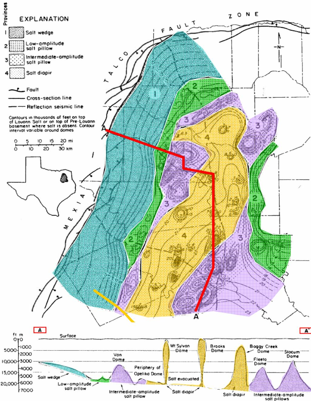
**Figure 10:** Structure map of the top of Louann Salt depicting the four salt provinces in the East Texas Basin. Red line represents the location of the cross-section. Yellow line is the approximate location of the northwestern portion of the 2D seismic line. [Modified from Jackson and Seni, (1983)]
