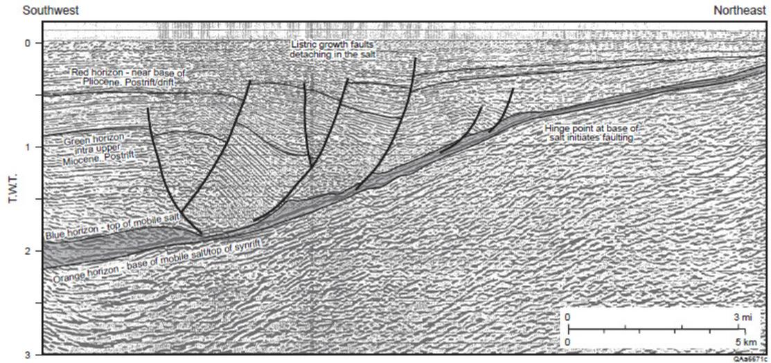
**Figure 50:** Listric growth faults in the Yemeni Red Sea detaching in salt and sliding basinward causing extension and rollover of the beds into the fault block, much like the listric faults in this study. [Modified from Heaton et al. (1995)]
