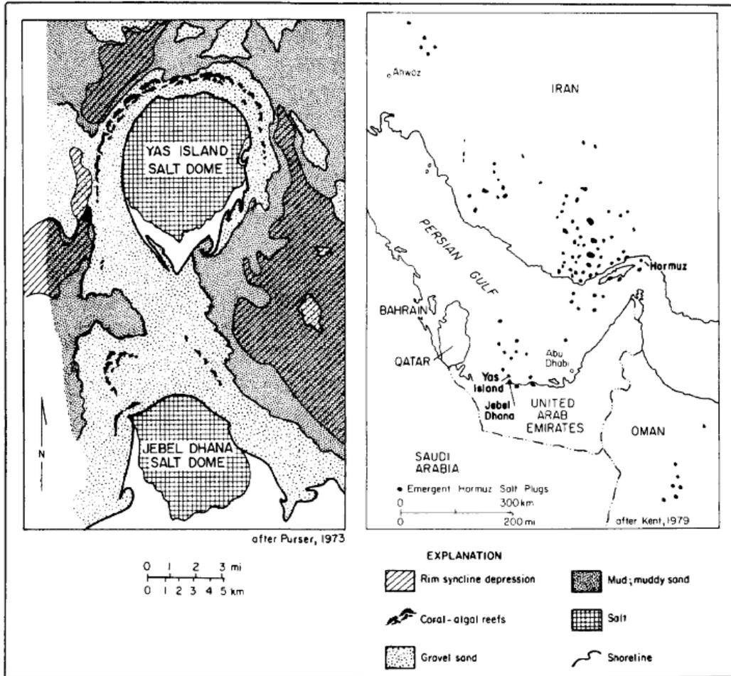
**Figure 51:** The Yas and Jebel Dhana salt domes in the Persian Gulf. Both are exposed at the surface and surrounded by a fringe of coral reefs with carbonate sands on their flanks forming a rim syncline (Seni and Jackson, 1983).
