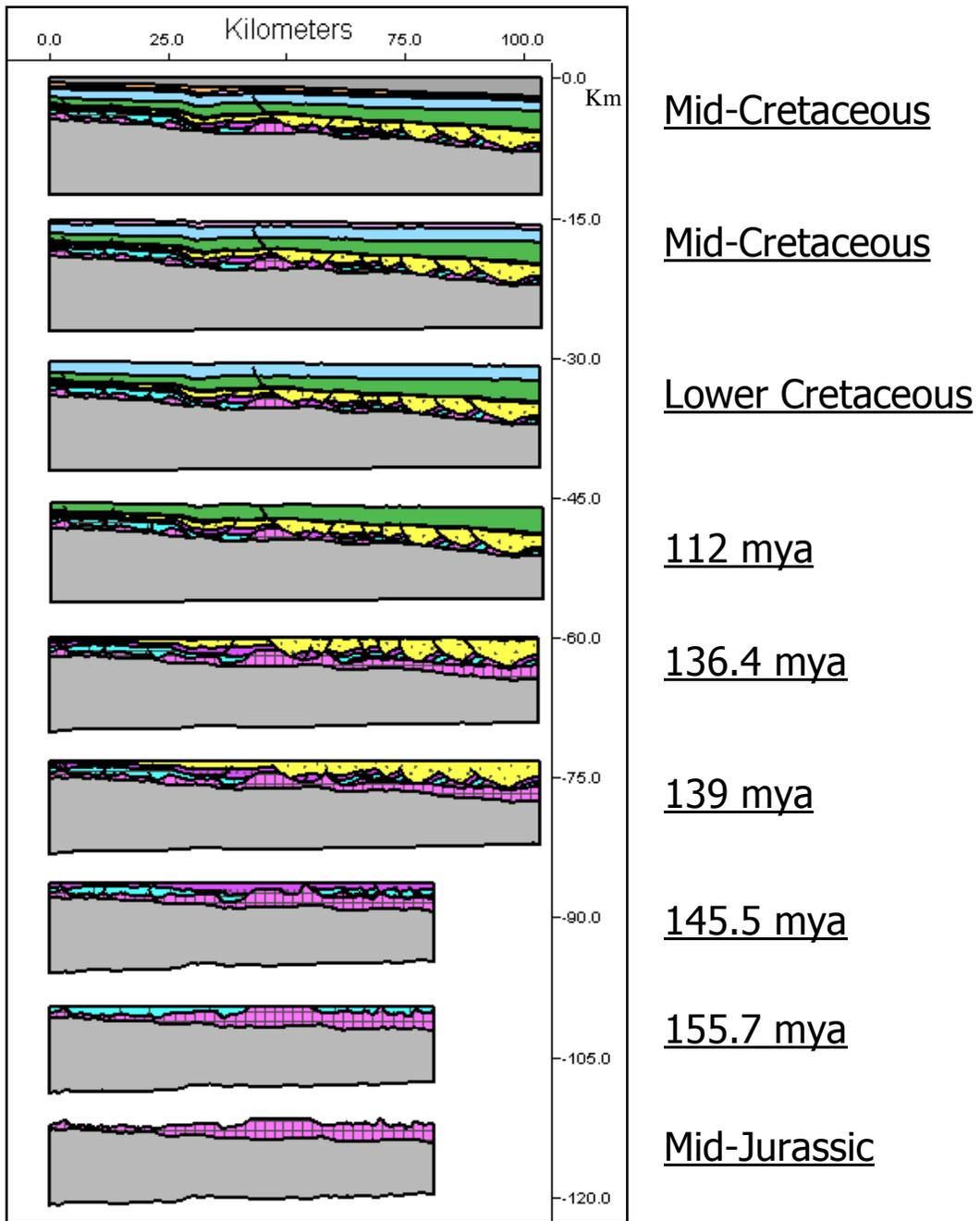
**Figure 47:** Complete LithoTect restoration of depth-converted 2D line through Freestone, Leon, and Houston counties in the East Texas Basin. Vertical exaggeration is 2:1. Refer to Figure 23 for stratigraphic column. Time in millions of years ago (mya).
