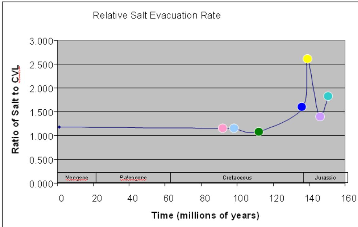
**Figure 34:** Ratio of Louann Salt to Cotton Valley Limestone. The Cotton Valley Limestone was used to compare to the thickness of salt because it is present in the same length as the salt, it is not lost down-dip off the line when the Bossier extension is restored.
