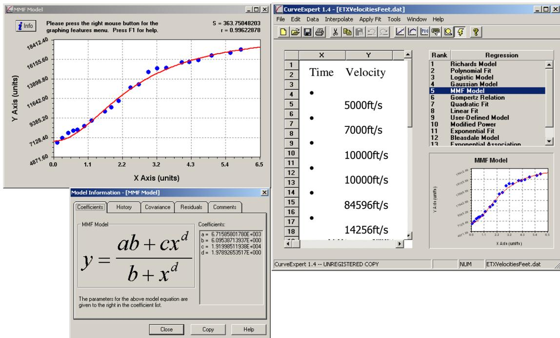
**Figure 20:** CurveExpert software that was used to do the velocity analysis and produce an equation for the best fit line along the values. The MMF model was the fifth closest fit, but was the only one that would work with the LithoTect software.
