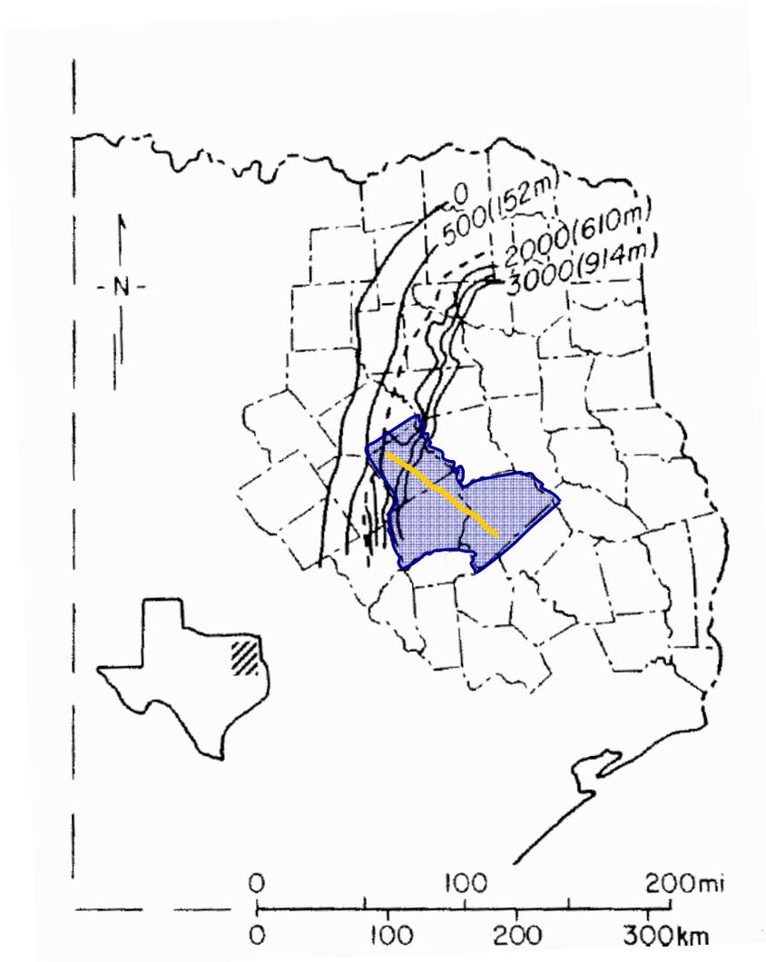
**Figure 41:** Isopach map of Smackover-Cotton Valley Limestone carbonate facies. Northwest of dashed line is an isopach of Smackover alone. Southeast of dashed line is a combined Smackover-Cotton Valley Limestone isopach. Study area in blue and 2D line in yellow. [Modified from Harris and McGowen (1987)]
