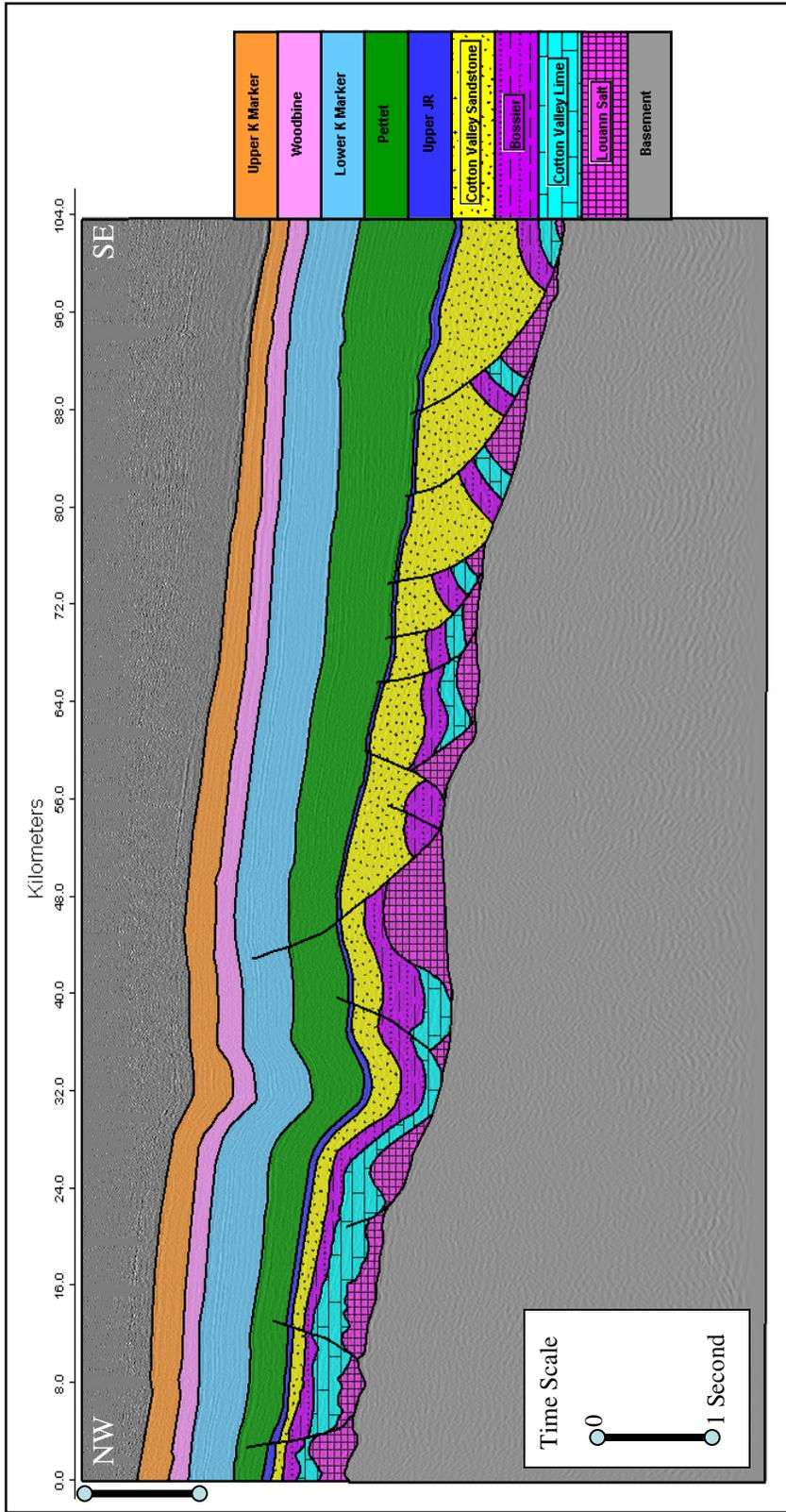
**Figure 19:** Time Interpretation supported by well data and 3D seismic in the area. Vertical exaggeration is 2:1. Courtesy of Seismic Exchange, Inc. and Marathon Oil Company.
