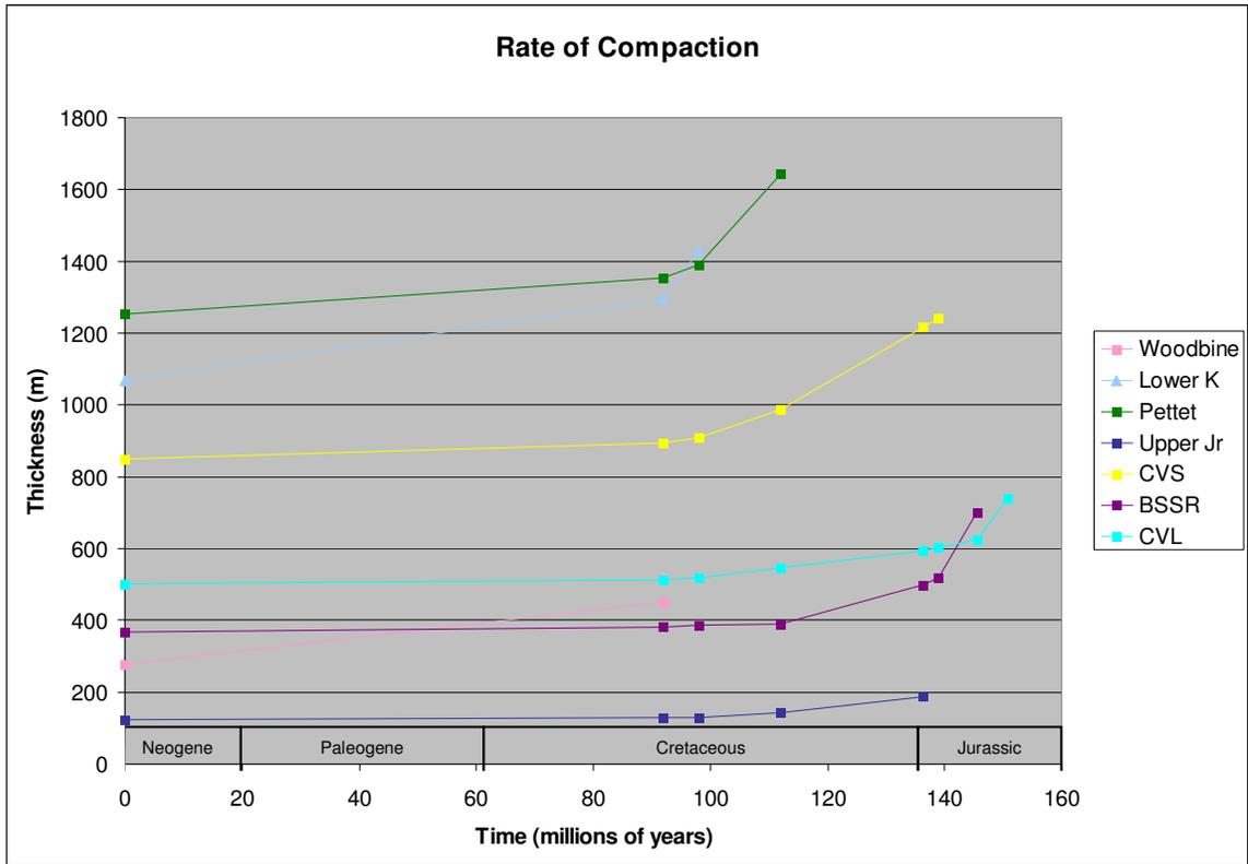
**Figure 38:** The rate of compaction over time for each formation.
