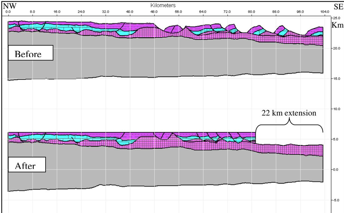
**Figure 31:** Before and after reconstruction of the Bossier Formation. Upon returning the Bossier to regional, it is obvious that the salt is thicker, and there was a significant amount of extension during Cotton Valley Sandstone deposition. Vertical exaggeration is 2:1. Refer to Figure 23 for stratigraphic column.
