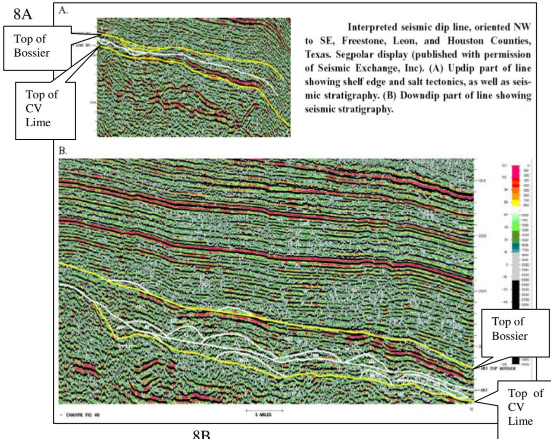
**Figure 8:** Klein and Chaivre's (2002) interpretation of the Bossier Formation. Figure 8A displays the seismic interpretation with the white line illustrating the stratigraphy within the Bossier. Figure 8B is an animation of the seismic interpretation showing that the mounded geometries represent basin floor fans. In this interpretation, the Cotton Valley Sandstone appears to have no gradational relation with the Bossier.
