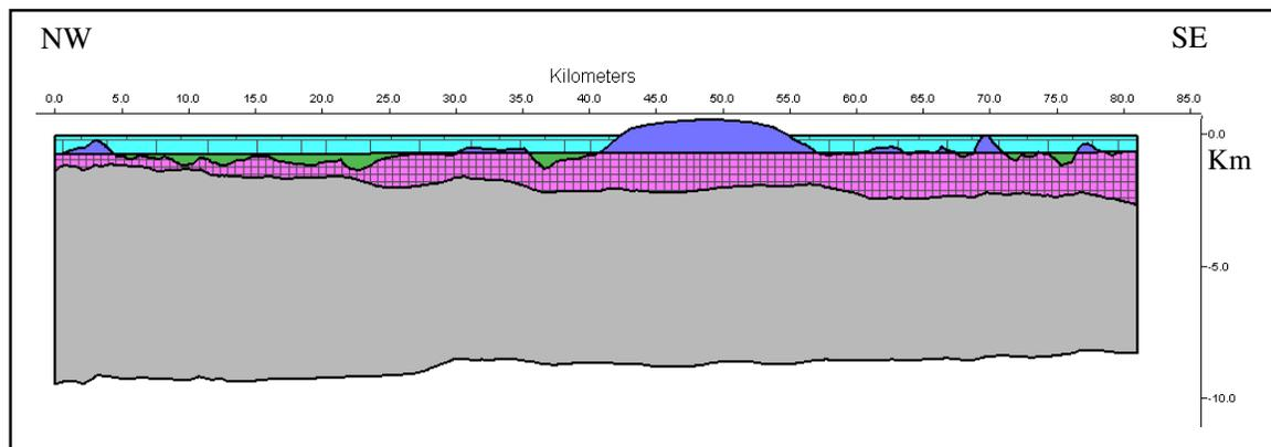
**Figure 35:** The areas of salt (dark blue) above the regional salt elevation should be equal to the Cotton Valley Limestone (green) below regional elevation. The dark blue salt has an area of 18.7 km<sup>2</sup> versus 8.9 km<sup>2</sup> of green Cotton Valley Limestone. Since the areas are not equal, this suggests that there was salt flow from out of plane. Vertical exaggeration is 2:1. All units are in kilometers.
