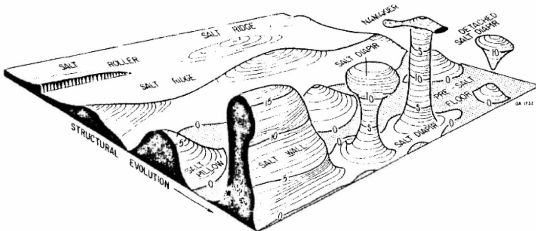
**Figure 11:** Evolution of salt features in the East Texas Basin. The oldest and most evolved structures are concentrated in the central most part of the basin (Jackson and Galloway, 1984).
