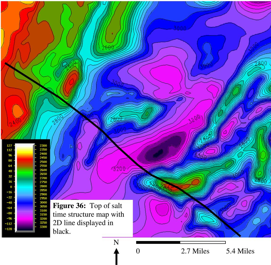
**Figure 36:** Top of salt time structure map with 2D line displayed in black.
