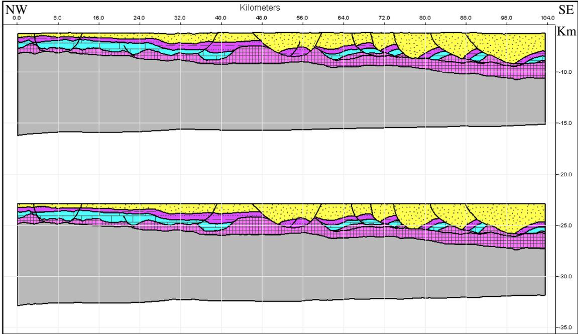
**Figure 29:** Before and after reconstruction of the Cotton Valley Sandstone. When the Cotton Valley Sandstone are returned to regional, there is slightly more salt added to the system, but there is no evidence of extension at this stage. Vertical exaggeration is 2:1. Refer to Figure 23 for stratigraphic column. All units are in kilometers.
