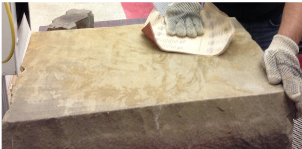
Figure 4.35: Both surfaces of the sandstone block is getting flattened using sandpaper.
