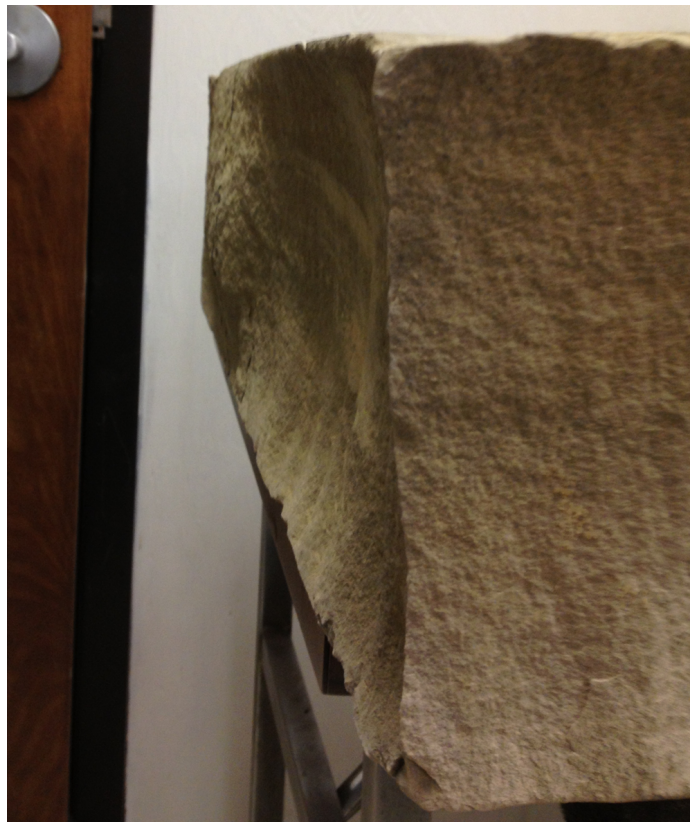
Figure 4.37: Side view of the sandstone block. It is not suitable for deploying well-side transducers.
