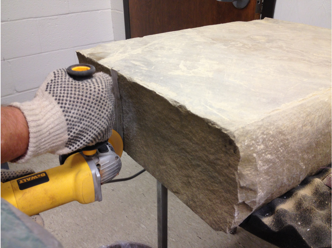
Figure 4.38: A "well" is constructed and aligned vertically. The second well is built at the other side of the rock.
