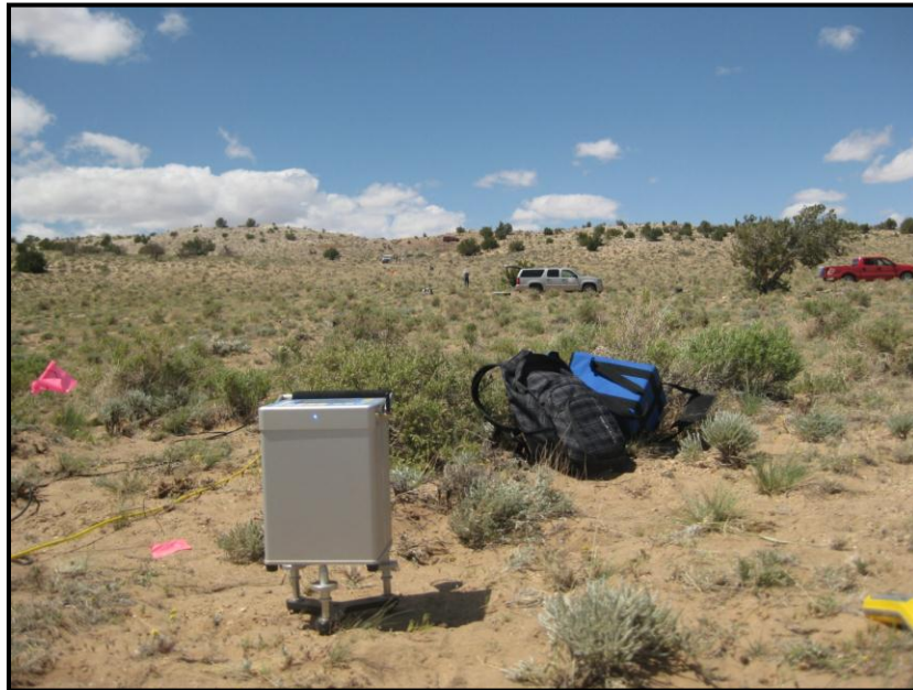
Fig. 3.2. Photo of Scintrex CG-5 relative gravimeter (gray box in foreground) at a gravity station at Meteor Crater. Rim of crater is in background (Photo courtesy of Eray Kocel).
