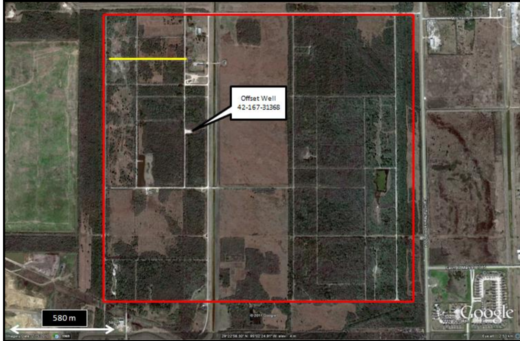
Fig. A.3. Google Earth image of area of study. Red box outlines extent of UHCC and yellow line represents extent of seismic reflection study. Callout points to offset well used in seismic to well log correlation.
