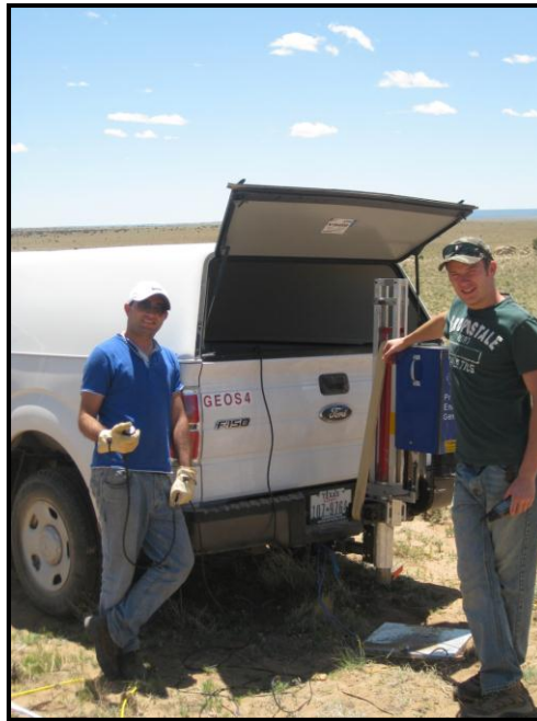
Fig. 1.1. Photo of seismic acquisition crew (author on right) using the weight drop mechanism on the rear of a pick-up truck as the source of the seismic acquisition. (Photo courtesy of Eray Kocel).
