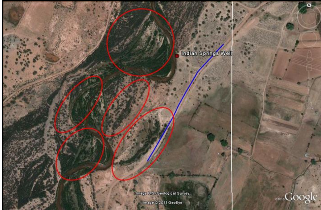
Fig. 4.28. Google Earth image of seismic study area. Blue and white lines denote extent of the Jemez Pueblo seismic line and the Indian Springs Fault Zone, respectively. The red circles bound ancient ox-bow lakes and river channels that make up the larger Jemez River channel system.
