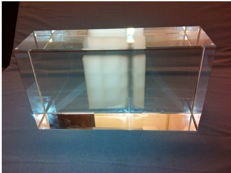
Figure 2.2: Glass model C11. The cloud inside the glass is the laser-etched fracture zone with 281 vertical fracture planes.
