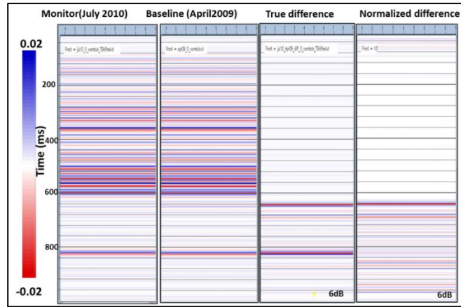
Figure 4.15: The normalized difference in the corridor stack can be generated by dividing the true difference by the RMS of the monitor panel. The true difference is the subtraction of baseline from the time-shifted monitor.
