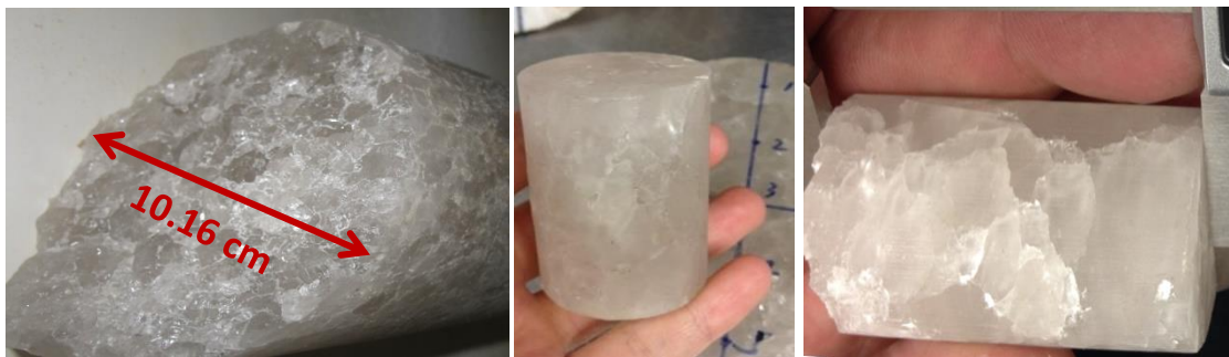
Figure 2.4 Salt cores from Bayou Corne, Louisiana. The left figure is the original 4-inch diameter salt core. On the middle (L1) and right (L2) are the 1 inch plugs for high pressure tests, which are cut from the salt core.
