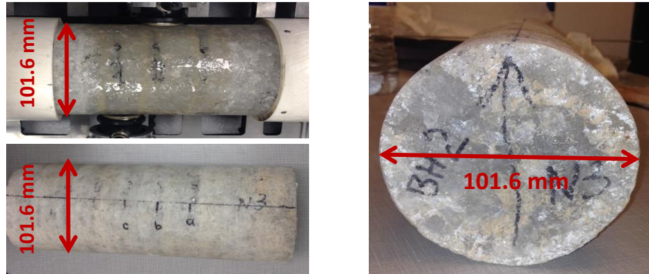
Figure 2.6 Salt cores from Hockley Salt Mine, Texas. The left two figures are: H4 and H5 from top to bottom. The right figure is a cross-section view of H5.
