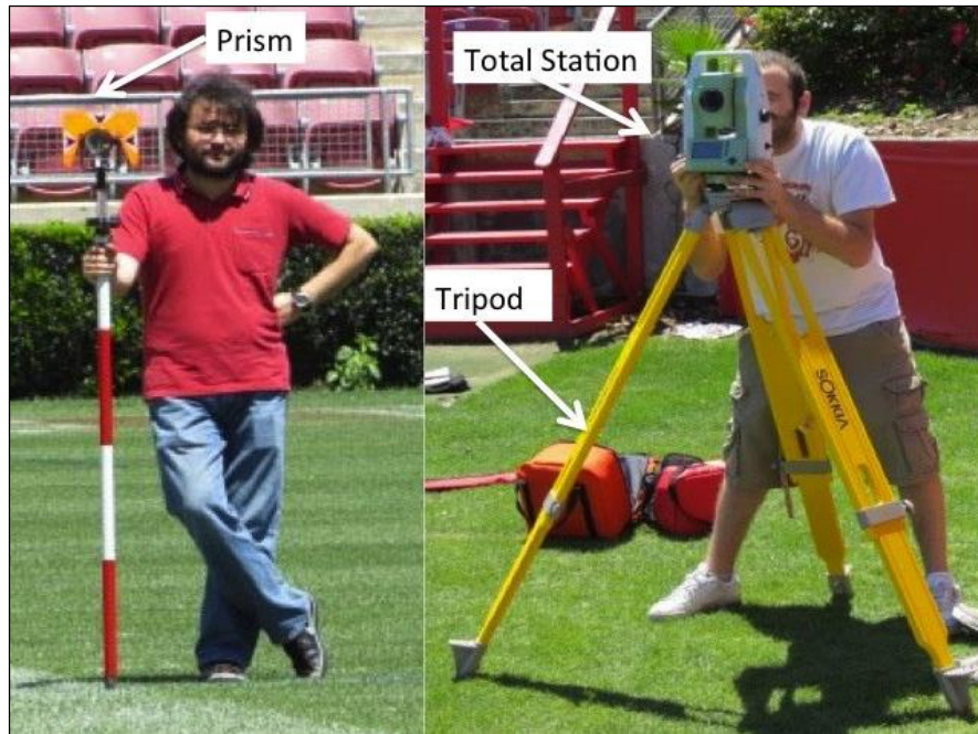
Figure 2.7. Element of the total station survey instrument.
