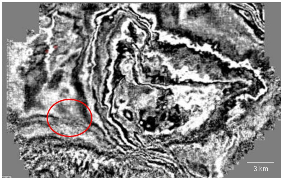
**Figure 3.4** – Time slice taken at  $t=1.5s$  from the Company B volume. The red circle is area where acquisition footprint can be seen.
