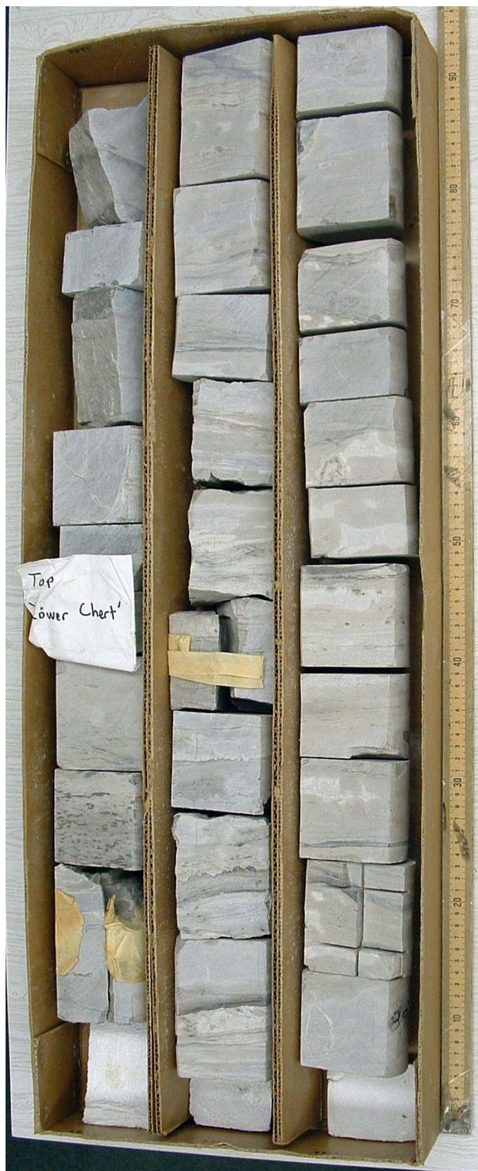
Box 11: 8885-93, 8894-8903, 8904-14 ft. 9/30 ft core recovered. 5 ft Carbonates at the top. Lower part is laminated chert and contains more stylolites.
