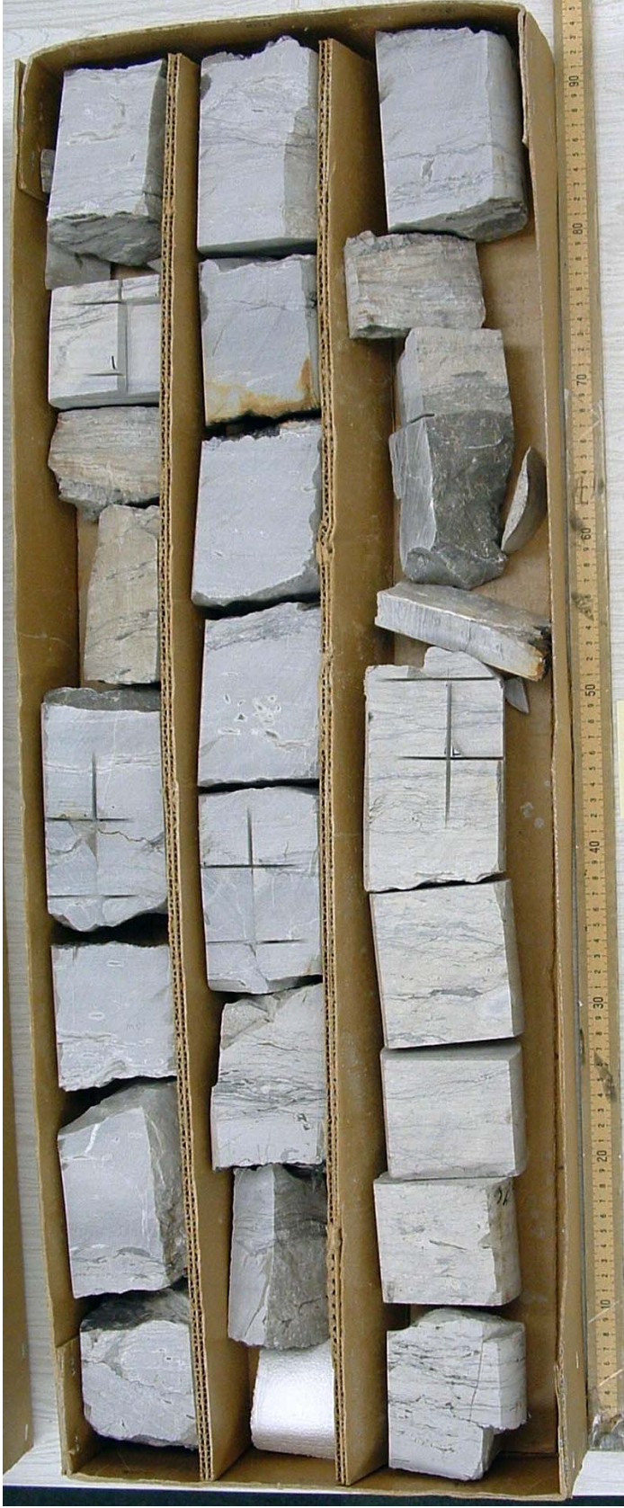
Box 15: 9004-10, 9011-17, 9018-25 ft. 9/19 ft core recovered. Laminated chert dominates. Some carbonates are present in dark color. Vertical veins developed at 2-3 cm spacing. Stylolites development is less intense than the lower interval.
