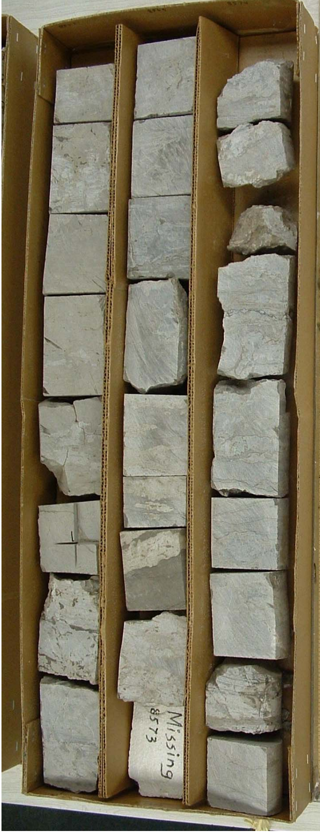
Box 5: 8557-64, 8565-73, 8574-81 ft. 9/25 ft core recovered. Brecciated chert and carbonates laminae. Stylolites developed. Induced fractures developed along stylolites. Stylolites teeth are 0.5-1.5 cm high. Lower part is carbonate.
