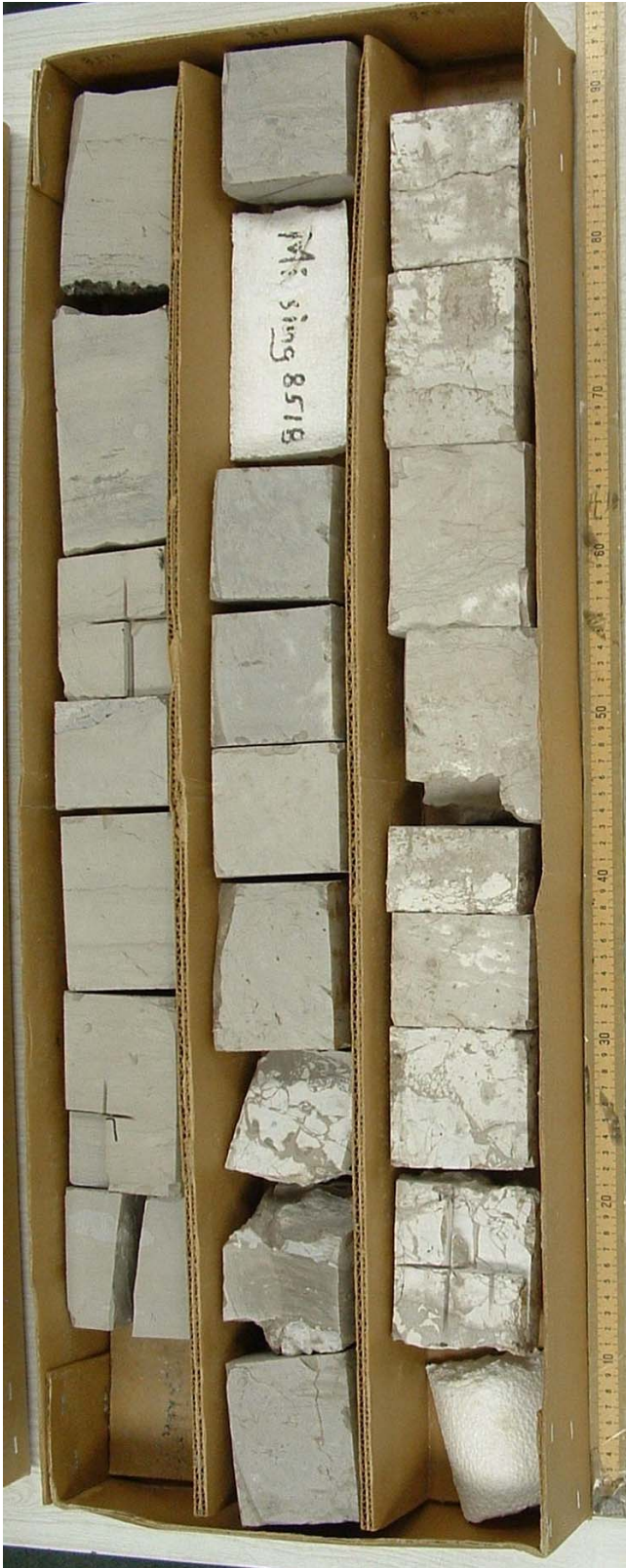
Box 3: 8510-16, 17-24, 25-32 ft. 9/23 ft core is recovered. 8510-8521: 5/12ft recovered, thick-bedded chert. 1 vertical fracture, dipping 80 degree, at 8516ft, partially filled with calcite. 8522-8532: 4/11 ft recovered, light color, brecciated chert.
