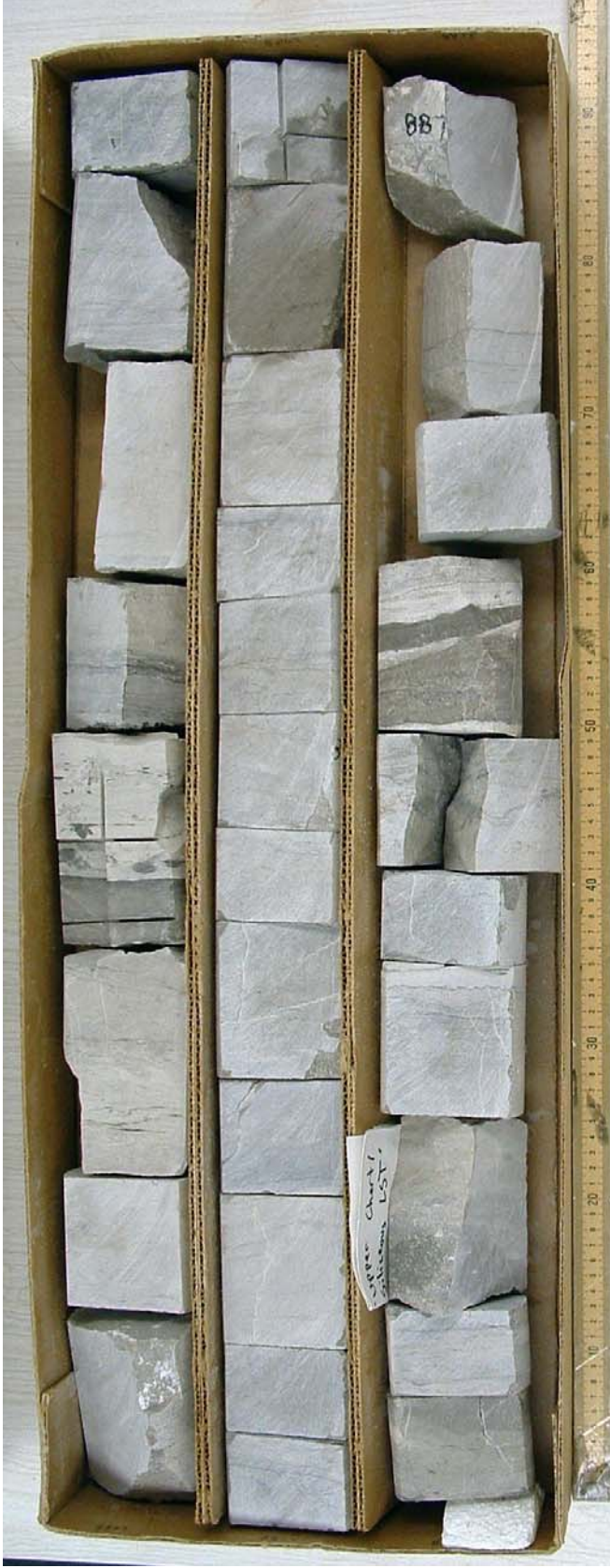
Box 10: 8855-62, 8863-74, 8875-84 ft. 9/30 ft core recovered. 8855-62 ft, limestone/chert mixture is present. Lower part is light-gray limestone.
