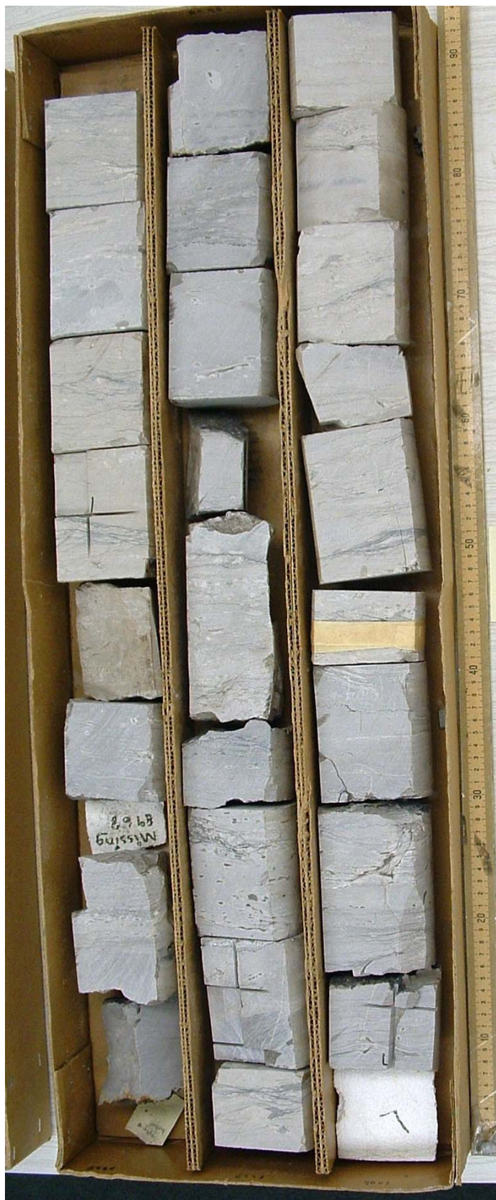
Box 14: 8976-84, 8985-93, 8994-9003 ft. 9/27 ft core recovered. Light gray, laminated chert and thick-bedded chert mixed. Stylolites developed with 0.5 cm high teeth. Carbonates nodules present.
