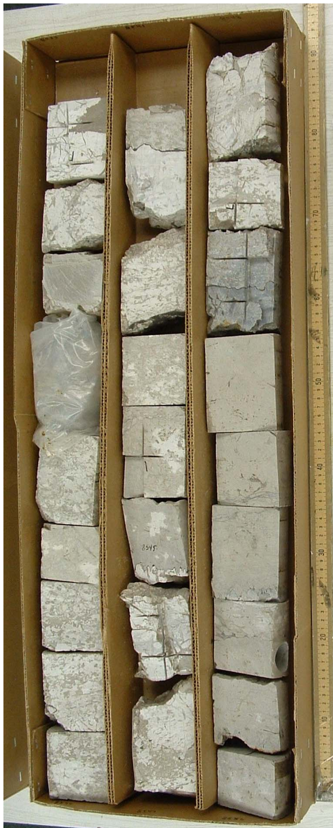
Box 4: 8533-40, 8541-47, 8548-56 ft. 9/24 ft core is recovered. 8533-8548: 7/16 ft core recovered. Brecciate, porous, cemented with carbonate mud. Stylolites are present with 0.5cm high teeth. Lower part (8549-8556): less-brecciated chert, fewer stylolites, less porous.
