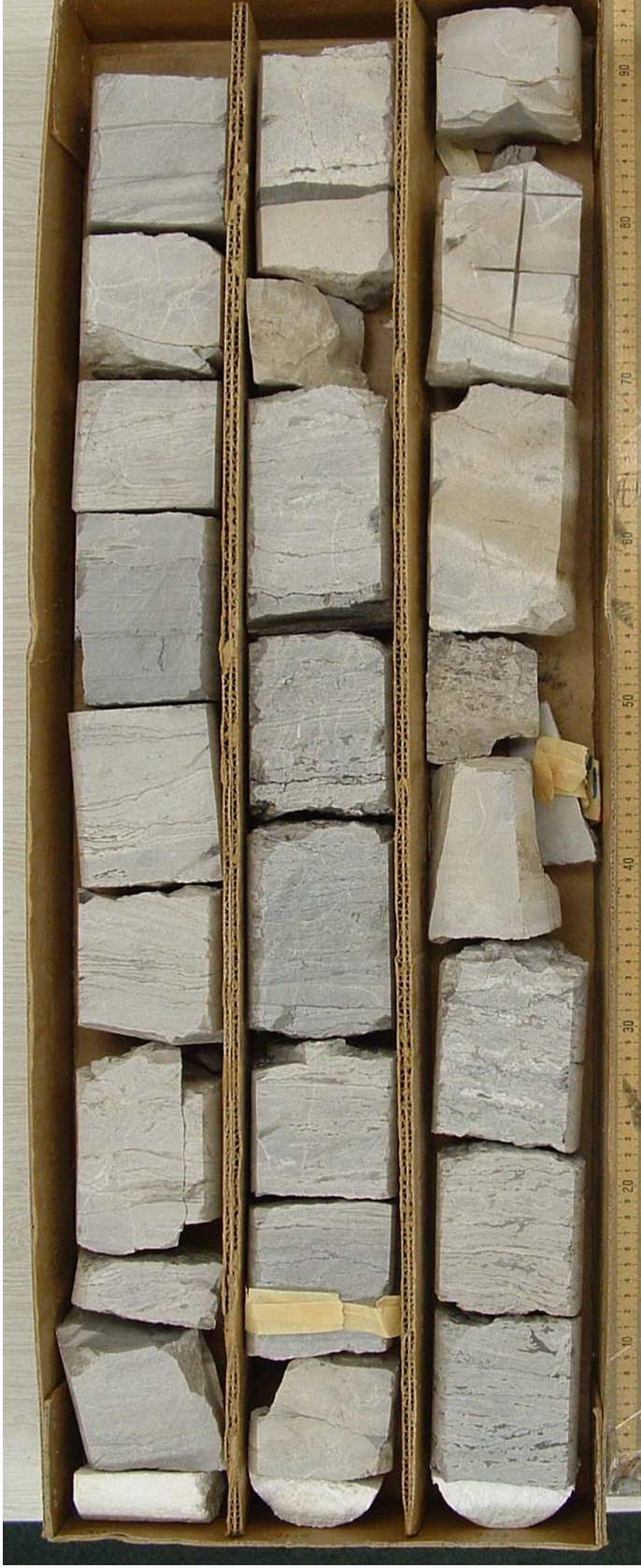
Box 18: 9099-9107, 9008-15, 9016-23 ft. 9/24 ft recovered. Laminated chert/carbonates dominate. Some thick-bedded chert is present. The light-color laminated chert is more permeable than dark ones, indicated by the absorption efficiency of water spray. Oil stains are seen along the stylolites, which might be conduit of fluid underground.
