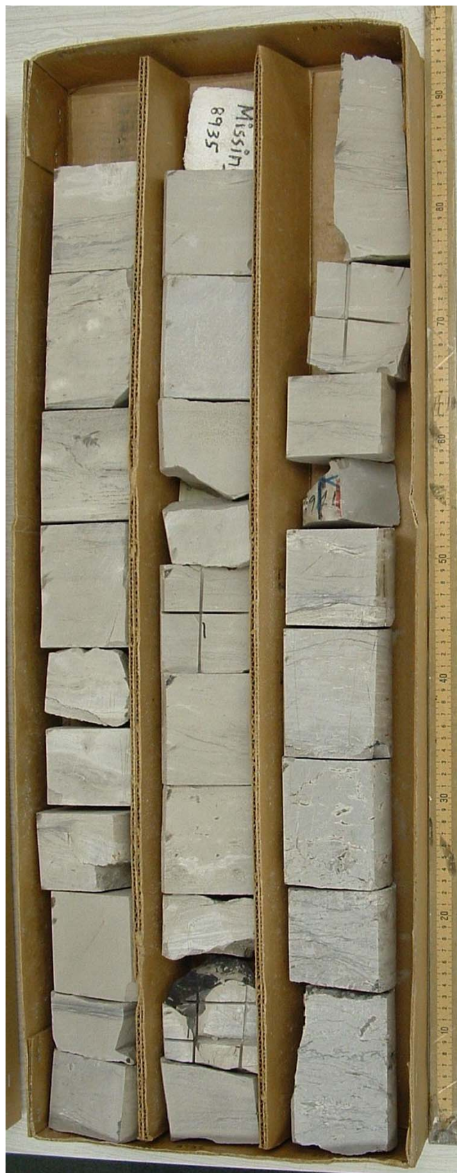
Box 12: 8915-25, 8926-36, 8937-45 ft. 9/30 ft core recovered. Thick-bedded chert is present with fewer stylolites. Clusters of calcite are present at the chert boundaries. One stylolite dips at 60 degree. It might be a sealed fracture or small fault. The stylolites are weak points. Many core breaks at stylolites. Laminated chert is present.
