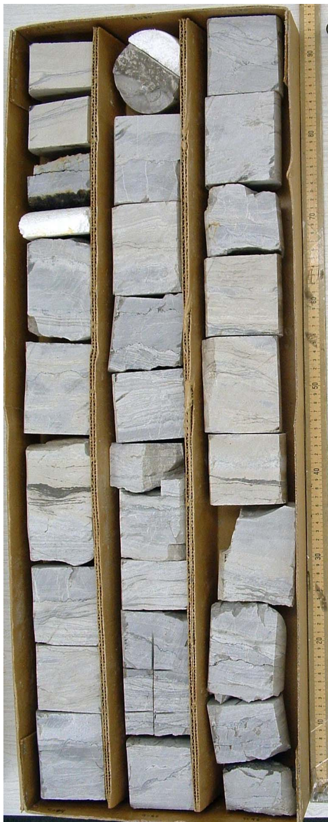
Box 17: 9056-9071, 9080-88, 9090-98 ft. 9 out of 42 ft recovered. Laminated chert and thick-bedded chert are present. Stylolites are common with a centimeters spacing. Veins are developed between stylolites and stop at stylolites. Veins are normally filled with calcite, which were originated from dissolution from stylolites.
