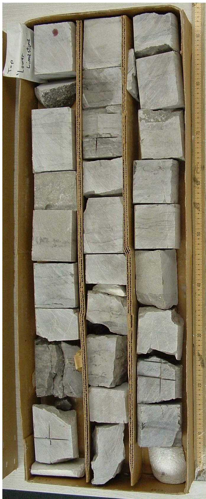
Box 9: 8826-34, 8835-45, 8846-54 ft. 9/28 ft core recovered. Limestone dominates. Some laminated chert is present. Horizontal bedding.
