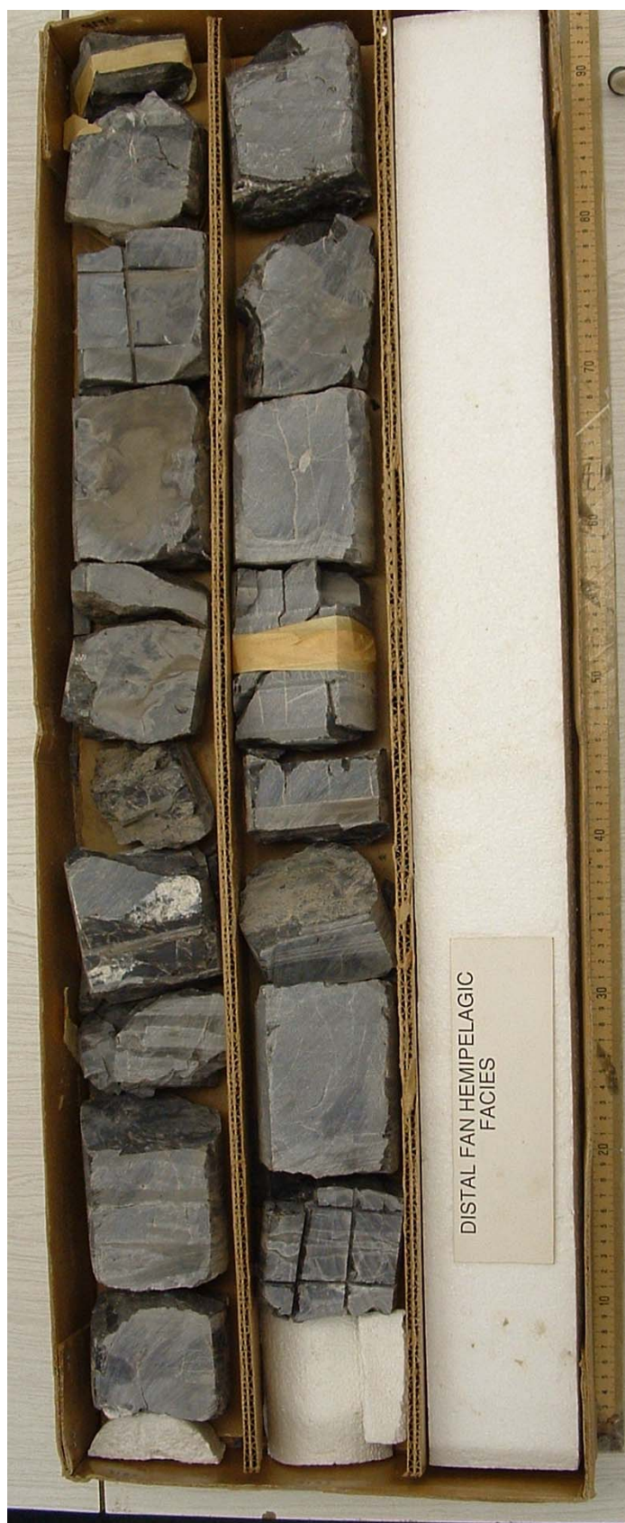
Box 21: 9176-9185, 9186-9183 ft. Dark, glassy chert, brittle, broken into pieces. Vertical veins developed in the beddings and stop at boundaries.
