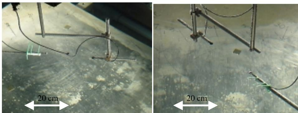
FIG. A.2. Beam pattern data collection setup in the acoustic (water) tank.
