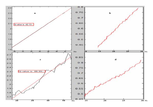
Figure 4.3 (a) is the noise-free Fourier amplitude spectral ratio compared to the correct spectral ratio (LnA1-LnA2). (b) is the amplitude spectral ratio line generated by CWT. (c,d) corresponding to (a) and (b) with Gaussian random noise added.
