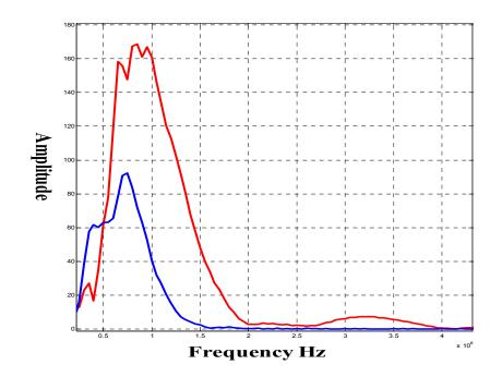
Figure 4.5 (a) is the amplitude spectrum of the signal (FFT), Red and blue lines are A wave and C wave, respectively.
