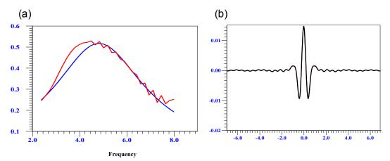
Figure 2.4 (a) The amplitude of the spectrum of the transient signal  $f_T(t)$  and corresponding adapted wavelet are presented. Red line: the optimal wavelet. Blue line: original signal. (b) The matched wavelet with zero degree phases.
