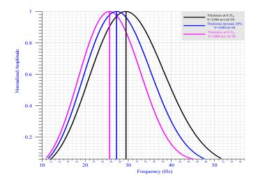
Figure 5.10 Comparison of the effect of a 20% thickness increase and 20% velocity decrease on peak frequency. (Vp from 2300 m/s to 1800m/s).
