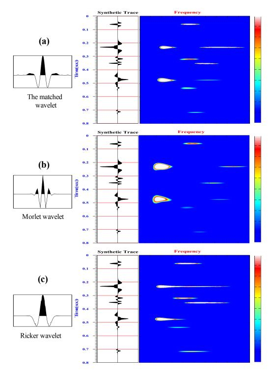
Figure 2.8 The results of time-frequency decomposition of the synthetic trace by using three different wavelets. (a) is the result of time –frequency using the matched wavelet, (b) is the result using the Morlet wavelet , and (c) is the result using the Ricker wavelet.
