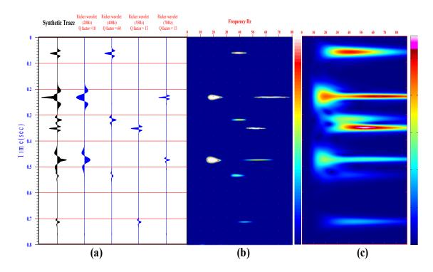
Figure 3.10 Comparison of results of application of spectral decomposition to a (a) synthetic seismic trace using (b) the hybrid wavelet transform and (c) continuous wavelet transform.
