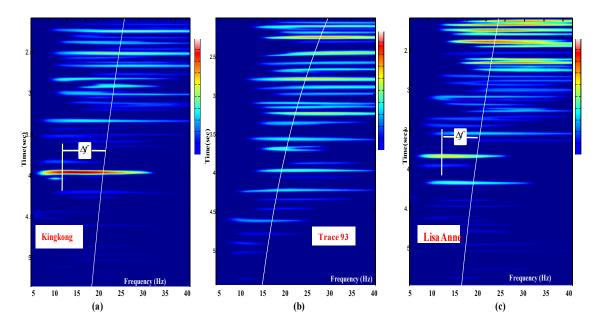
Figure 6.5 Time-frequency gathers of seismic traces. (a) is the time-frequency gather of the seismic trace located at the KingKong well. (b) is the time-frequency gather of the seismic trace 93(blue line Figure 6.4). (c) is the time-frequency gather of the seismic trace at the Lisa Anne well. The white line is a curve fit of the peak frequency background trend. Note that large low-frequency anomalies appear at the target sand location.
