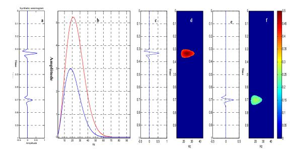
Figure 4.1 (a) and (b) are two synthetic events and their amplitude spectral, the red line is the first event and blue line is second event. (cdef) are signals and corresponding time-frequency decompositions with CWT.
