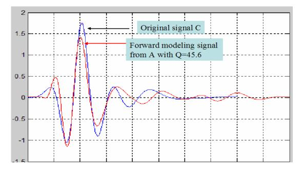
Figure 4.8 the blue line is the transmission wave C. red line is the wave generated by the reflector wave A with forward modeling.
