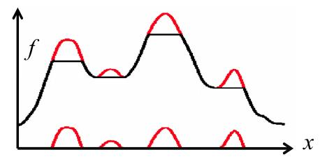
Figure 3.7 Top-hat transforms to extract local extreme value, the above line is a function containing the local maxima (red line segments), and the lower part is the top hat transform results.
