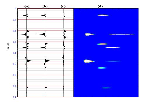
Figure 3.11. (a) is an original synthetic trace. (b) is an reconstruction of the signal by using HWT results. (c) is a residual between the original and reconstructed signal. (d) is the time frequency spectral of HWT.
