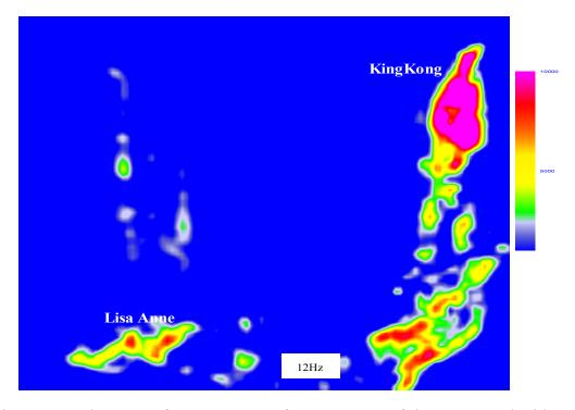
Figure 6.13 The 12 Hz frequency map of RMS energy of the target sand with a window horizon +/- 35 ms. The gas-containing sand was very accurately outlined at this frequency and the quality of gas-containing sand was also indicated by magnitude of energy spectrum.
