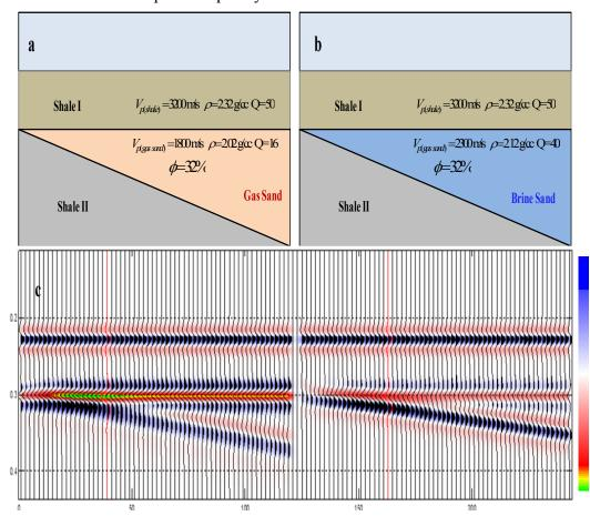
Figure 5.8 The geology model and its synthetic seismic traces. The red traces indicate at one-half wave length thickness location
