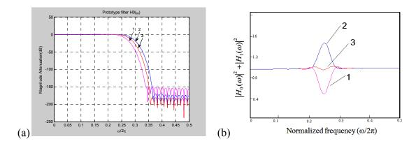
Figure 2.2 (a) The frequency responses of three different  $H_0(\omega)$ . (b) Amplitude distortion as function of degree of overlap between analysis filters.
