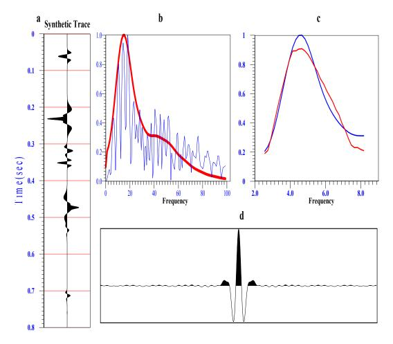
Figure 2.7 (a) The synthetic seismic trace. (b) The normalized Fourier frequency spectrum (blue line) and the power spectral density (red line) of the signal. (c) The modulated spectrum of the signal and corresponding adapted wavelet. Red line: the optimal adapted wavelet. Blue line: the synthetic signal. (d) The optimal adapted matched orthogonal wavelet.
