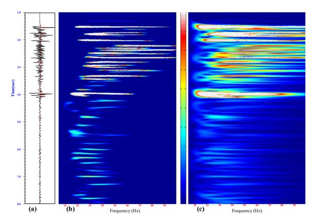
Figure 3.12 Comparison of results of application of spectral decomposition to a (a) real seismic trace using (b) the hybrid wavelet transform and (c) continuous wavelet transform.
