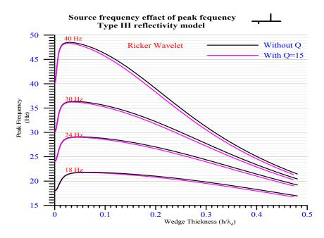
Figure 5.6 Source frequency effect of peak frequency for four different input Ricker wavelets with peak frequencies of 18Hz, 24Hz, 30Hz, and 40Hz.  $r_1$ = -0.18,  $r_2$ =0.2.
