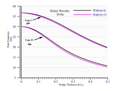
Figure 5.4 Peak frequency versus thickness for two different type of reflectivity models with the same frequency source wavelet (Ricker wavelet 30Hz). The initial peak frequencies are different as the thickness starting from zero. The initial peak frequency of type I is  $\sqrt{3/2} f_0$ , which is higher than that of original source wavelet.
