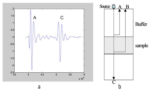
Figure 4.4 (a) The wave A is reflected from the top of the sample and C is the transmitted wave. (b) The schematic diagram of the measurement.
