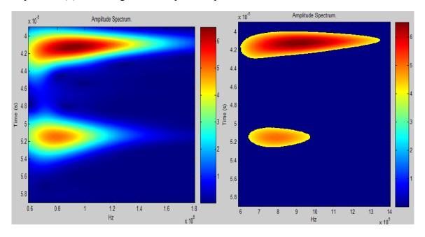
Figure 4.7 (a) CWT time-frequency spectrum of the signal, (b) the threshold window filter applied to (a).
