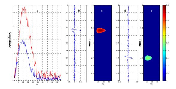
Figure 4.2 (a) is the amplitude spectra of two synthetic events with noise, the red line is the first event, and the blue line is second event. (bcde) are signals and their time-frequency decompositions with CWT.
