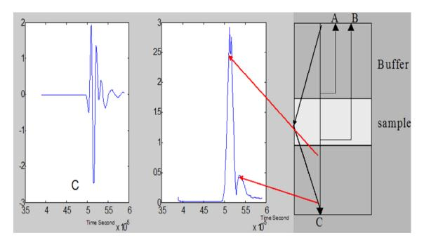
Figure 4.6 (c) is the amplitude spectrum of Hilbert transform, note the second peak of amplitude. (d) is the diagram of the possible path of C wave.
