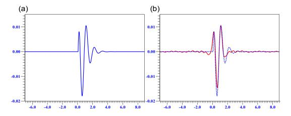
Figure 2.5 The transient  $f_T(t)$  and corresponding adapted wavelets are presented. (a) The transient signal. (b) Dashed blue line: the optimal adapted wavelet matched by the method described in this paper. Solid red line: original signal.
