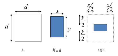
Figure 3.5 Morphological erosion of an image
