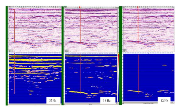
Figure 6.11 The results of the three common frequency sections (bottom) by the hybrid wavelet transform with Inline 5529 seismic profile.
