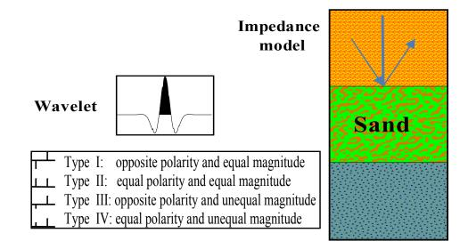
Figure 5.1 Three-layer "boxcar" model and its four types of the reflectivity series.
