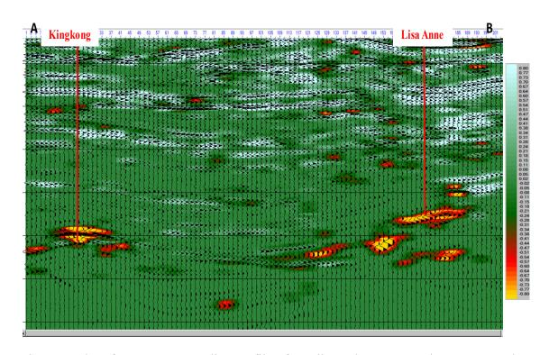
Figure 6.6 low frequency anomalies profile of AB line. The orange color represents large negative peak frequency anomalies.
