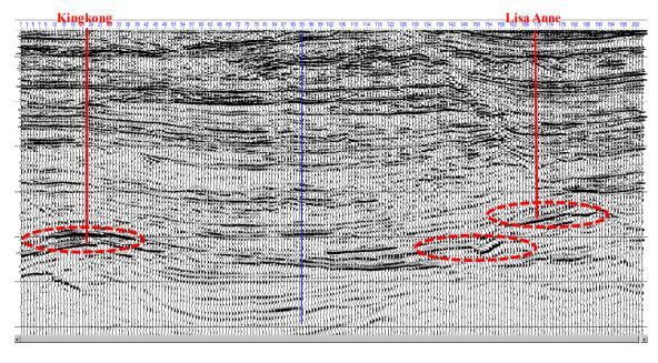
Figure 6.4 A seismic profile line AB that crosses the wells KingKong and Lisa Anne. The blue line marks trace 93 where no frequency anomaly appears.
