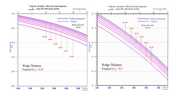
Figure 5.7 Velocity variation effect for peak frequency of type III reflectivity model with the fixed thickness place. The left is wedge thickness fixed at 0.25 wavelengths. The right is wedge thickness fixed at 0.5 wavelengths.
