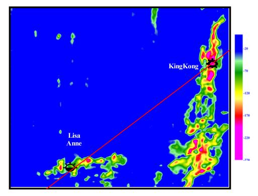
Figure 6.7 Sum of negative frequency anomalies of 2D map of target sand horizon with window at  $\pm$  50 ms.
