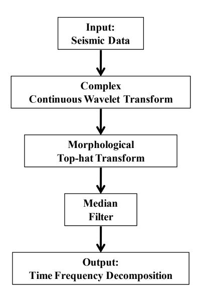
Figure 3.9 The flowchart for spectral decomposition using the hybrid wavelet transform.
