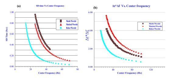
Figure 2.9 (a) The standard deviation in time versus the center frequency. (b) The uncertainty product  $\Delta t^*\Delta f$  versus the center frequency.
