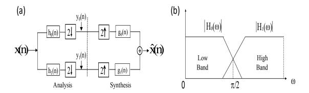
Figure 2.1 (a) The quadrature mirror filter bank. (b) Typical frequency magnitude response of analysis filters.
