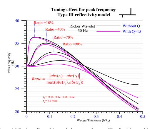
Figure 5.5 Tuning effect of the peak frequency for type III reflectivity model. In this example, the  $r_1$  values are -0.18,-0.12,-0.06, to -0.02 and the  $r_2$  is fixed at 0.2, The maximum value of peak frequency shifts toward thicker beds as the difference of the two reflectivity coefficients increases. Note the systematic suppression of peak frequency value as  $r_1$  influence relatively decreases when Q taken into account (pink line).
