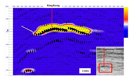
Figure 6.12 Local seismic trace profile (wiggle) and 12 Hz common frequency profile (colored background) near the KingKong well. Note that the arrow points the gas water contact boundary where the phase reversal occurs.
