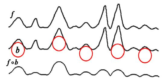
Figure 3.6 (Top, a) a scan line of function. (Middle, b) positions of rolling ball for opening. (Bottom,c) Results of opening.
