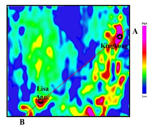
Figure 6.3 RMS amplitude of a 2D map of target sand horizon with a window around the horizon +/- 25 ms. Note that both KingKong and Lisa Anne exhibit the amplitude anomalies.
