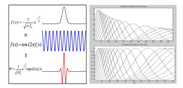
Figure 3.1 Construction of the Morlet wavelet as a cosine curve modulated by a Gaussian in the time domain (left) and its dictionary in the frequency domain (right up) and after normalization (right down).
