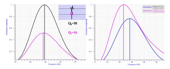
Figure 5.9 Left (a) is the frequency response of the two signals with only changing Q values. The right (b) is the frequency response of brine sand velocity Vp=2300 m/s and gas sand velocity=1800 m/s.
