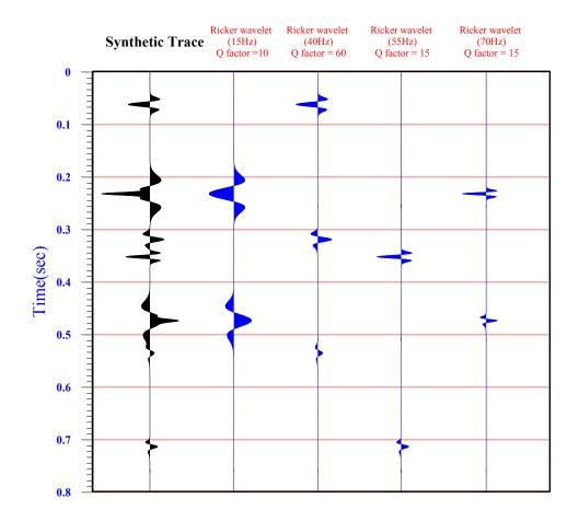
Figure 2.6 Synthetic trace composed of Ricker wavelets with different center frequencies. Q values are specified at the top.
