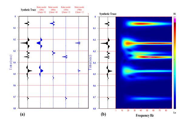
Figure 3.3 (a) Synthetic trace comprised of Ricker wavelets with different center frequencies, wave propagation attenuation was included. (b) Time-frequency distribution of synthetic trace by the continuous wavelet transforms.
