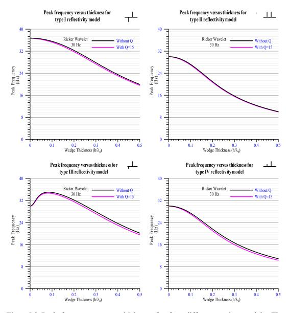
Figure 5.3 Peak frequency versus thickness for four different wedge models. The pink line shows the peak frequency location of the convolution model as a function of thickness with Q=15, the black line shows the peak frequency without attenuation consideration.
