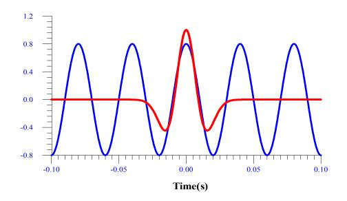
Figure 3.2 The center frequency of a Ricker wavelet (red line) is approximated by matching to the function  $\cos(2\pi f_c t)$  (blue line).  $f_c = 25Hz$  provides the best fit and is taken as the center frequency of the wavelet.
