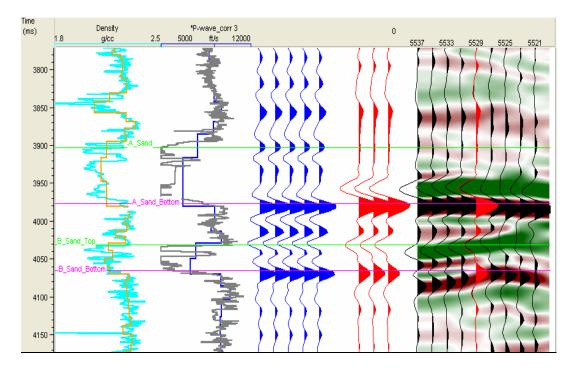
Figure 6.10 Density log, sonic log, synthetic trace, correlation trace and seismic section at KingKong well.
