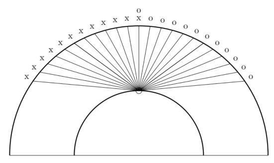
Schematic diagram of a common midpoint (CMP) source-receiver configuration in a spherical geometry. At far offsets, ray paths will not be able to reach the CMP location without transmitting through a lower boundary. The Cartesian normal moveout equation only holds for flat layers, it must be modified to represent the travel-time pattern in spherical geometry.
